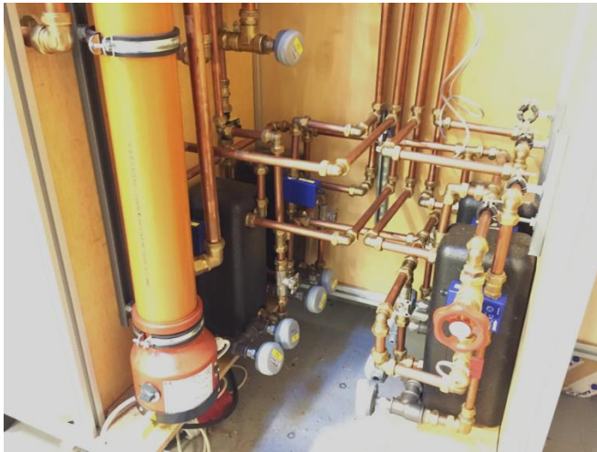
Figure 27 The heat exchangers emulating the heat emitters in a heating system (left). The actuators of the heating system (right).
