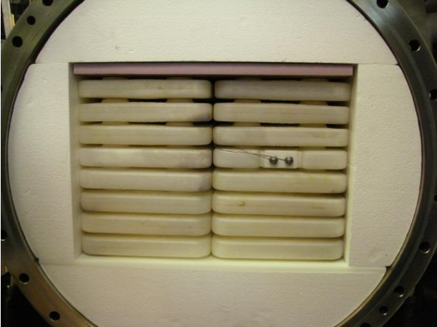
Figure 55: Position of the instrumented PCM capsule in the tank as viewed from the outlet.
