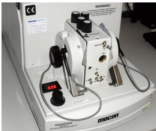
Figure 27: Mocon® AQUATRAN™ Model 2 on left. Schematic view of measurement principle on right.
