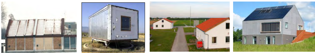
Figure 1: Examples of different types of full scale test facilities (left to right): facility for façade field testing, outdoor test cell, test buildings for energy use analysis and facility for in-use testing.
