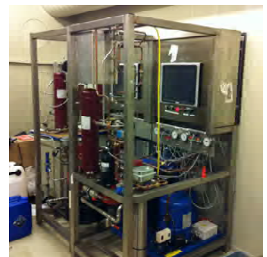
Test of heat pumps.
