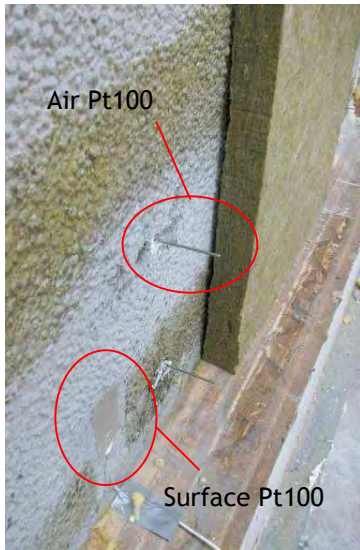
Left: Pt100 for air chamber and surface Pt100 installed below the insulation layer. Right: Distribution of air Pt100 in the air chamber.
