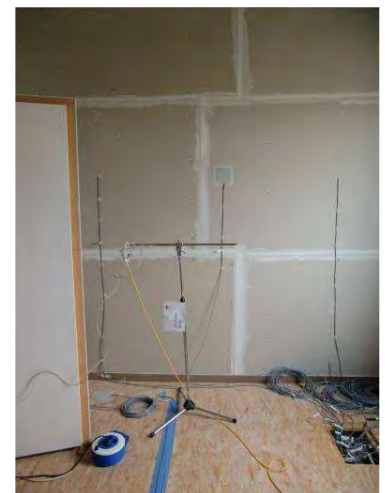
Radiation and temperature sensors on a measurement room in KUBIK
