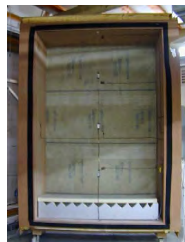
Semi Hot Box fitting a wall measurement bay in order to measure the overall U-value
