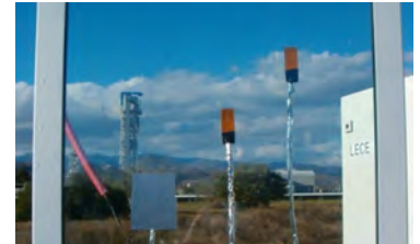
Pt100 used for surface temperature measurements
