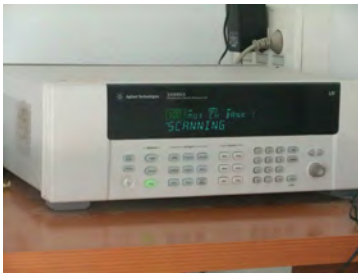
HP Agilent 34980A data acquisition system for logging and controlling the PASLINK tests.
