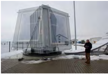
The calorimetric facades and rooftops testing facility under rotation.
