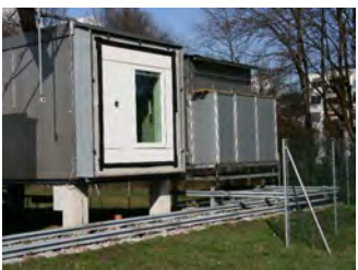
Test cell and Cold-Box in parking position
