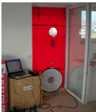
Airtightness test (blower door) in experimental houses.
