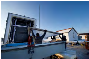
The calorimetric facades and rooftops testing facility during the mounting of a specimen.
