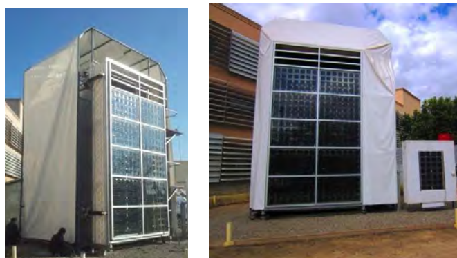
Figure 2. LOT test facility protected from solar radiation effects
