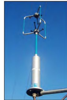
3D ultrasonic anemometer
