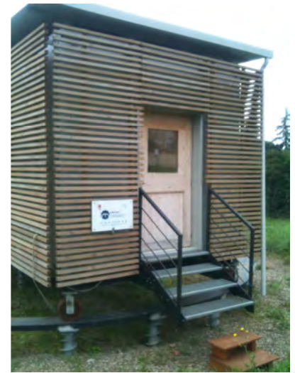
The test cell in wood with the external wooden solar screening.
