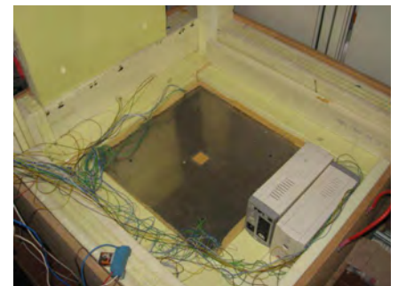
Calibration test of a heat flux tile.
