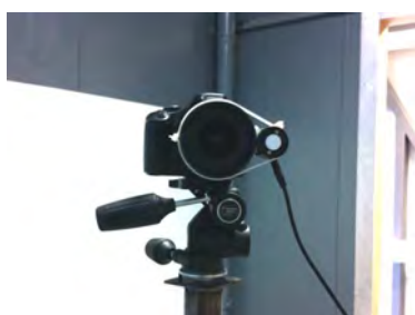
Canon Eos D450 for luminance measurements with separate illuminance sensors
