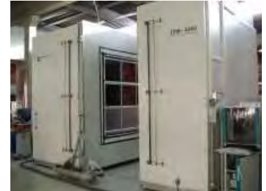
Test of building components in hot box.
