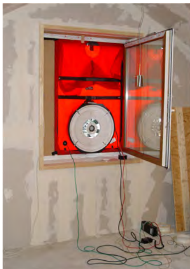
Blower Door device in attic
