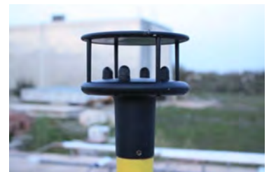
Used anemometer. Gill WindSonic 3
