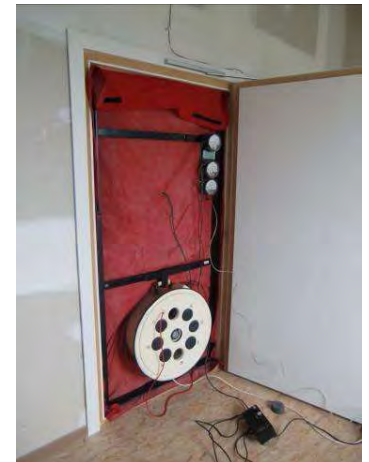
Air tightness test being performed in a measurement room in KUBIK
