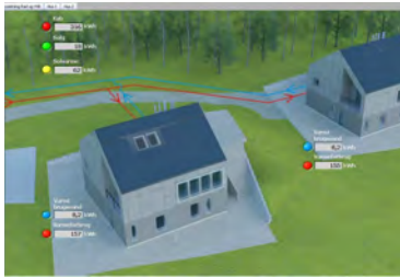
District heating for EnergyFlexHouse.
