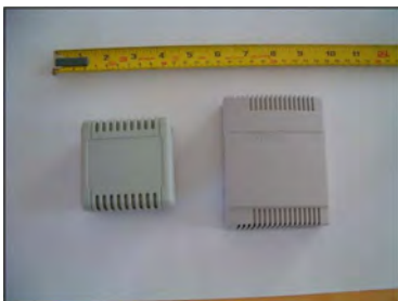
Installed indoor air temperature (left) and relative humidity sensors (right)
