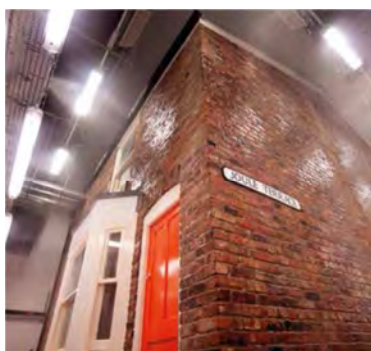
A wide range of boundary conditions can be placed on the structure including wind and rain
