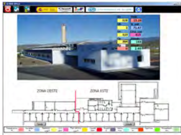
SCADA C-Ddl PSA: Main screen that shows instantaneous meteorological measurements
