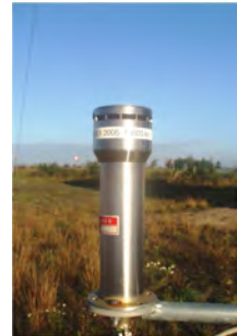
2D ultrasonic anemometer
