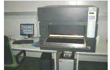
Heat flow meter apparatus (according to EN ISO 8301)
