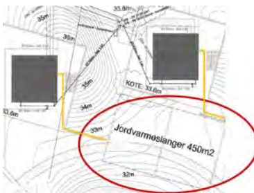
Area with ground source heat exchangers for the ground coupled heat pumps in EnergyFlexHouse.
