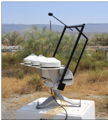
Devices measuring solar global and diffuse, and longwave radiation
