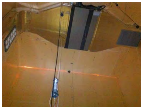
Figure 7. Position of thermocouples to measure the air
