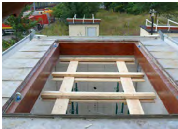
ILARGI: Frame for roof samples.
