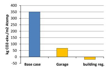
Figure: Module A1-5 compared to additional impact due to underground garage, and reduced impact due to insulation reduction if the house should only have complied with current energy norms in the Swedish building regulation.
