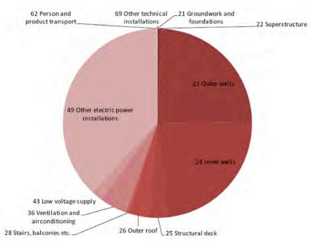
Embodied CO<sub>2eq</sub> (EG) emissions in materials and components distributed according to NS 3451:2009
