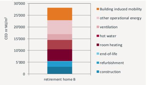
Figure 1: Contribution to the primary energy demand, non renewable, from the construction, operation and induced mobility for the rest home B.
