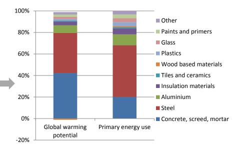
*Distribution between construction materials and operational energy for the reference study period of 50 years*  *Contribution from the life cycle of construction materials divided into different types of building materials.*
