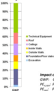
Figure 5: Contribution of the different construction elements divided into 7 different building cost groups to the primary energy and GWP related indicators covering the stages of production, replacement and end-of life treatment of the materials.
