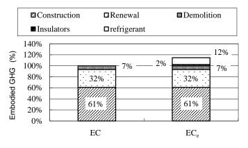
Fig.4 Embodied GHG due to insulators and refrigerants (Chillers) [1]
