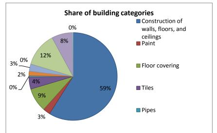
*Figure 2: Contribution of building categories to the total weight of installed materials.*
