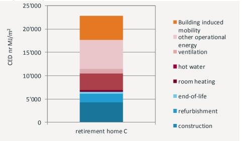
Figure 1: Contribution to the primary energy demand, non renewable, from the construction, operation and induced mobility for the retirement home C.
