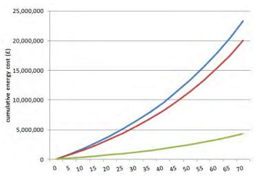
Cumulative energy costs for operating three equivalent commercial building designs over a 70 year period. Comparable assumptions on energy use have been made. The performance of the low carbon building is indicated with a green line. This building's operational costs were reduced by 75%, while its embodied greenhouse gas emissions were less than half compared to the other two buildings. Source: Best Foot Forward
