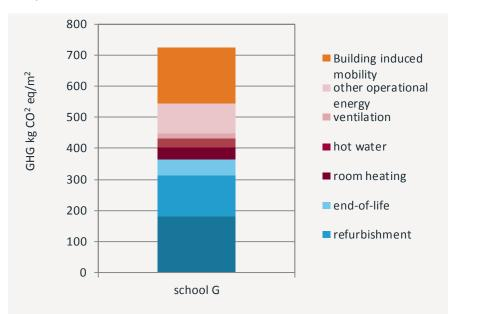
Figure 2: Contribution to the global warming potential from the construction, operation and induced mobility for the building school G.
