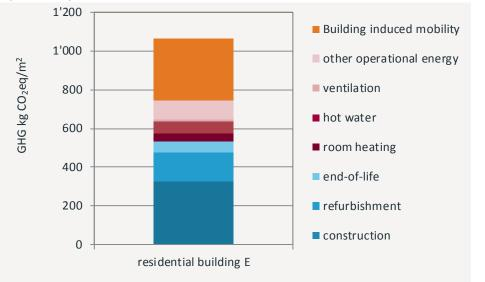
Figure 2: Contribution to the global warming potential from the construction, operation and induced mobility for the residential building E.
