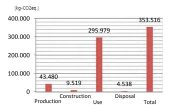
*Figure 1: Total amount of CO2eq emission by life cycle stage for Timber framed house*
