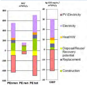
Figure 3: Distribution between construction materials and operational energy for the whole life cycle of the building.
