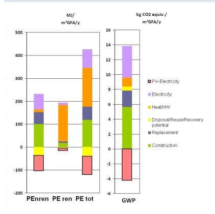
Figure 3: Distribution of shares between construction materials related impacts and operation related impacts considering the whole life cycle of the building.
