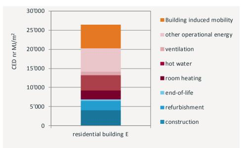
Figure 1: Contribution to the primary energy demand, non renewable, from the construction, operation and induced mobility for the residential building E.
