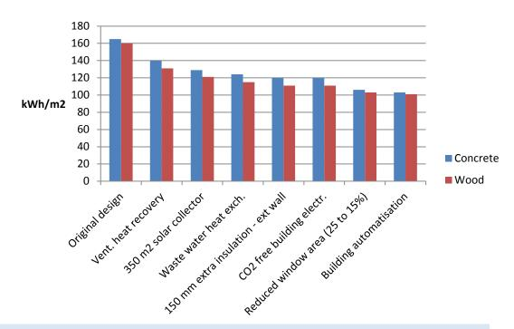
First the initial early design was modeled and operational energy use and GWP was calculated. After that an optimisation process was initiated, trying out different potential improvement measures with the goal to gain understanding about key improvement measures if to reach as low operational energy use and as low GWP as possible in the final design.
