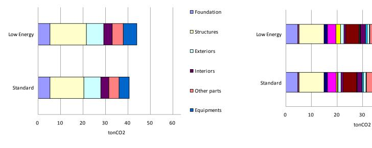
Fig.6 Comparison of CO2 (classification by parts) Fig.7 Comparison of CO2 ((classification by materials)
