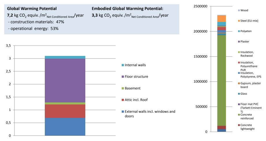
Figure 1: Contribution from the construction materials divided into 5 different building elements (kg CO2e/Net Conditioned Area/year). The impacts related to replacements of materials in the operation phase are not expressed here.
