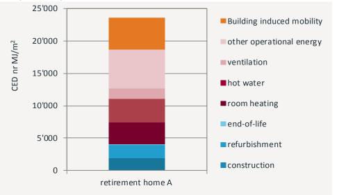
Figure 1: Contribution to the primary energy demand, non renewable, from the construction, operation and induced mobility for the retirement home A .
