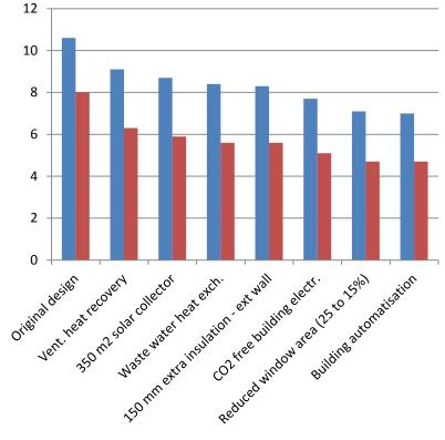
The figure above shows the final suggestion of improvement measures after the optimisation process and the approximate possible reduction of CO2e emissions that could be targeted.
