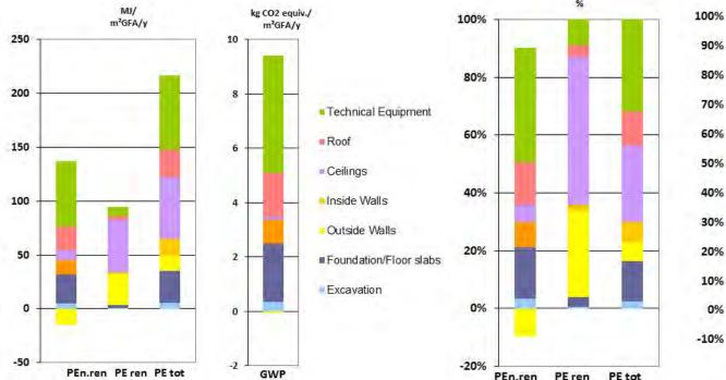
Figure 5: Contribution from the construction elements for the construction stage and end-of life treatment of the materials divided into 7 different building cost groups, replacements also included.
