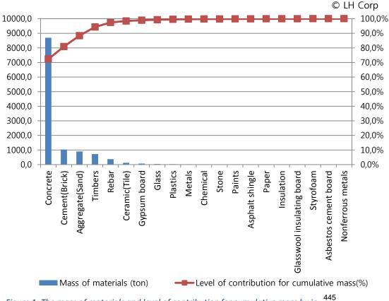
Figure 1: The mass of materials and level of contribution for cumulative mass by in <sup>44</sup> putted materials for multi-family residential building
