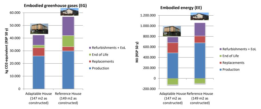
Notice: Results are given as totals for a reference study period of 50 years. The refurbishment scenarios for both houses entails the rearrangement of an inner wall, rearrangement of kitchen area and construction of 55 m2 additional space following the original design of the house.
