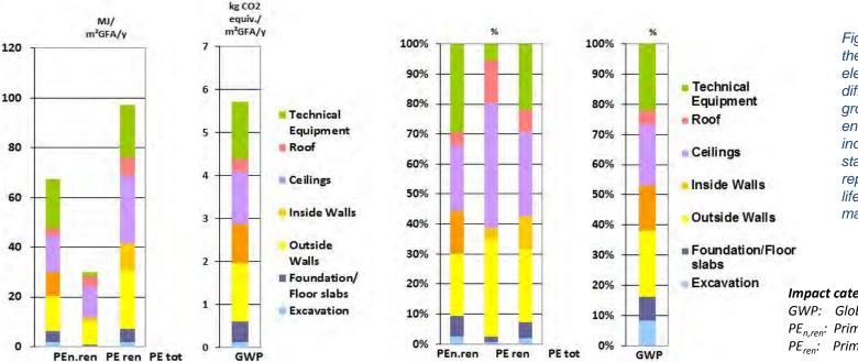
Figure 5: Contribution of the different construction elements divided into 7 different building cost groups to the primary energy and GWP related indicators covering the stages of production, replacement and end-of life treatment of the materials.
