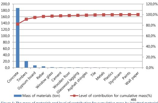
Figure 1: The mass of materials and level of contribution for cumulative mass by inputted materials for timber framed house
