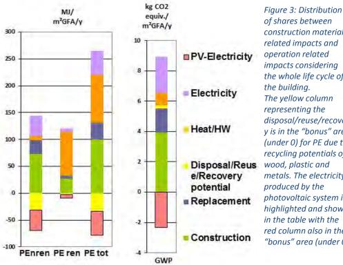
of shares between construction materials related impacts and operation related impacts considering the whole life cycle of the building. The yellow column representing the disposal/reuse/recover y is in the "bonus" area (under 0) for PE due to recycling potentials of wood, plastic and metals. The electricity produced by the photovoltaic system is highlighted and shown in the table with the red column also in the "bonus" area (under 0)
