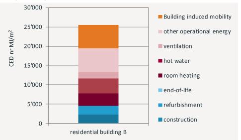
Figure 1: Contribution to the primary energy demand, non renewable, from the construction, operation and induced mobility for the residential building B.
