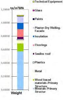
*Figure 1: Distribution of construction materials - production phase*
