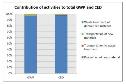
*Figure 3: Contribution of material production, transportation, and waste management to total GWP and CED.*
