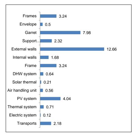
The recurring embodied energy represents the primary energy consumption related to the maintenance and/or refurbishment of some building components and technical installations.
