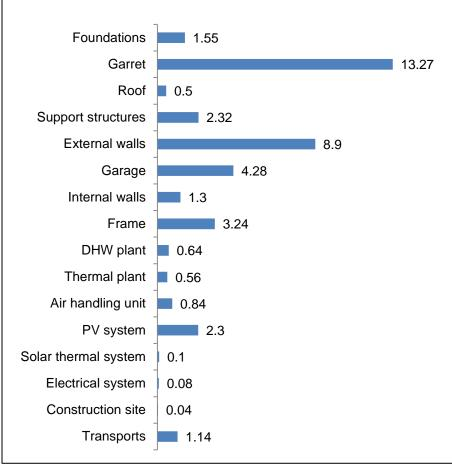
Embodied energy in the building elements for the production phase [MWh/y]
