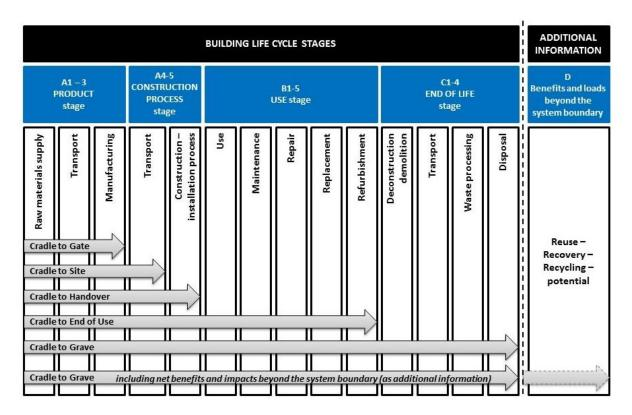
Figure 1-11: Overview of the various existing system boundary types using the respective modules of building life cycle model developed by the group CEN TC 350 (EN 15978:2011). (Balouktsi & Lützkendorf, 2016)
