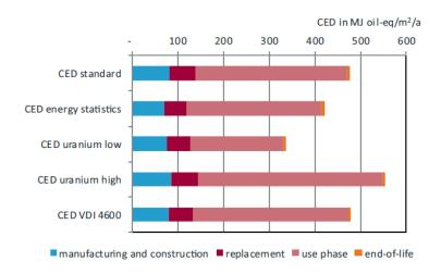
Figure 1-12: Cumulative energy demand of the life cycle of the building Rautistrasse in Zürich, differentiating between manufacturing and construction, replacement, use and end of life of the building (Frischknecht et al. 2015).
