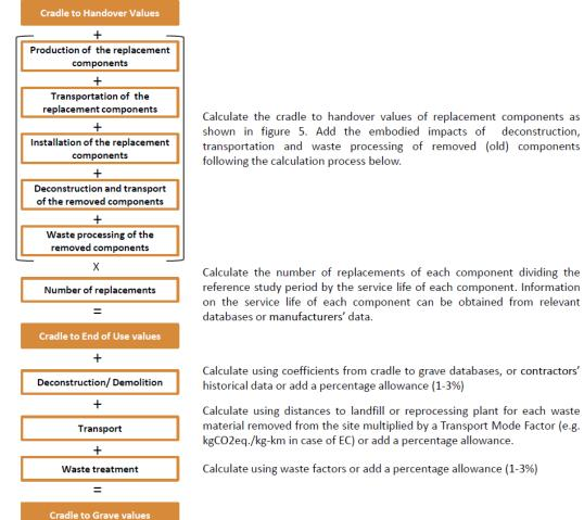
**FIGURE 7:** Typical process to calculate cradle to handover values of embodied impacts
