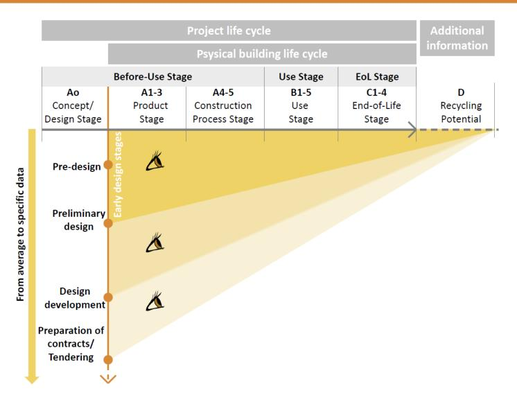
**FIGURE 2:** Relationship between project life cycle and building life cycle. The designer should consider the entire building life cycle in all phases of the Ao (Concept/Design) project stage – from the early design stages up to the final integration into contracts/tendering
