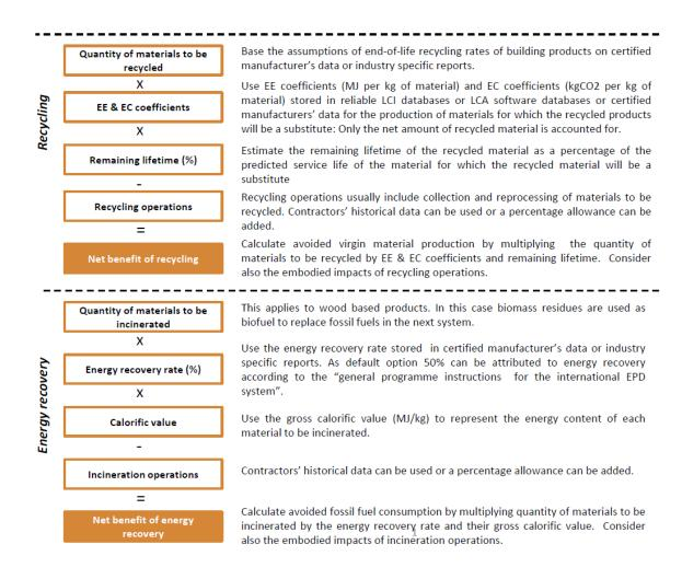
FIGURE 9: Typical process to calculate net benefits of recycling and energy recovery
