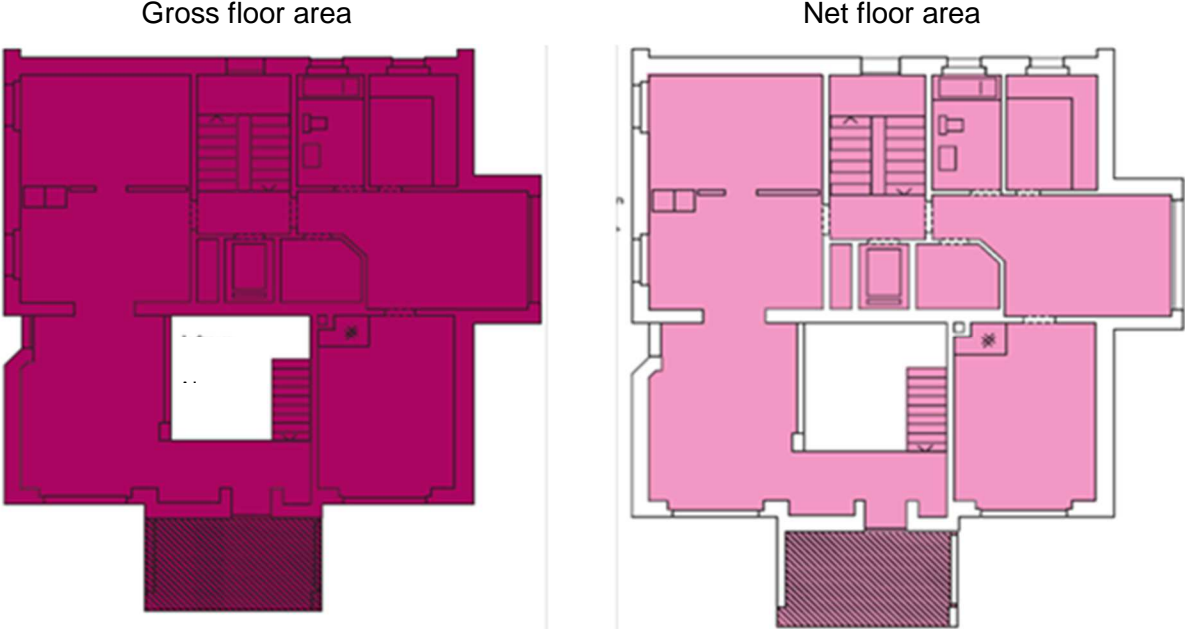
Figure 8 Illustration of (conditioned) gross floor area and net floor area. Hatched areas: Non conditioned exterior gross and net floor area respectively
