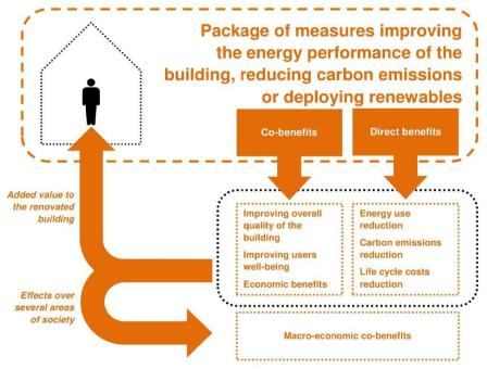
Some of the co-benefits whose connection with specific renovation measures have been identified are: -Thermal comfort -Natural lighting and contact with the outside environment -Improved indoor air quality -Reduction of problems with building physics -Noise reduction -Operational comfort -Reduced exposure to energy price fluctuations -Aesthetics and architectural integration -Useful building areas -Safety (intrusion and accidents) -Pride, prestige, reputation -Ease of installation
