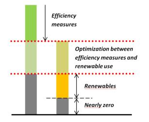
Figure 1 – Concept for an optimized combination of energy efficiency measures and renewable energy measures in building renovation with a nearly-zero energy and emissions target (Geier S., Ott W.).
