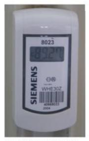
Figure 24: The electronic heat cost allocator
