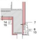
Figure 17: Construction detail D4 Entrance detail. Insulation under the first floor slab (on the ceiling of ground floor) in contact with unconditioned space.
