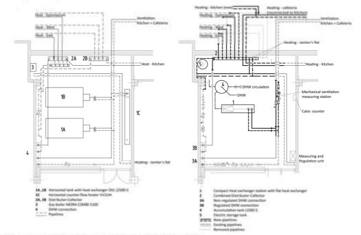
Figure 18: Schema of the boiler room before and after the renovation. [1]
