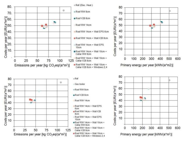
Figure 17: Comparison of cost effectiveness of energy efficiency renovation measures for the Portuguese Case Study for the BITS: electric heater (top) and gas boiler (bottom), as well as related impacts on carbon emissions and primary energy use
