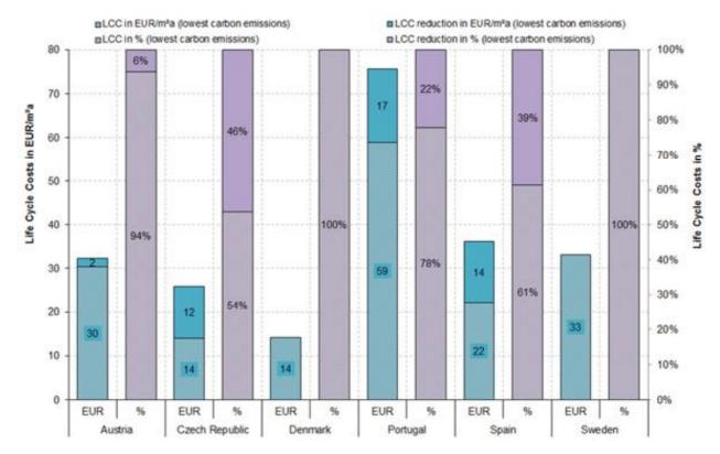
Figure 3: Life Cycle Cost reduction potentials of the six Case Studies. The absolute reduction potential (blue column) and the relative reduction potential (purple column) are presented as values between the reference case and the renovation package which achieves the highest carbon emissions reductions.
