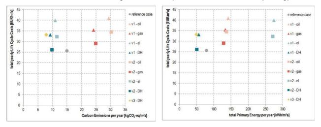
Figure 26: Life Cycle Costs in comparison with carbon emissions (left chart) and total Primary Energy (right chart) of the Case Study "Backa röd", Sweden
