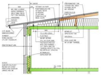
Figure 6: Cross section of exterior wall and roof construction.
