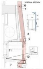
Figure 14: Construction detail D2 & D3. Vertical window section.
