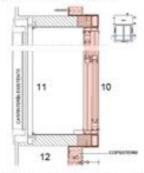
Figure 15: Construction detail D2 & D3. Horizontal window section.
