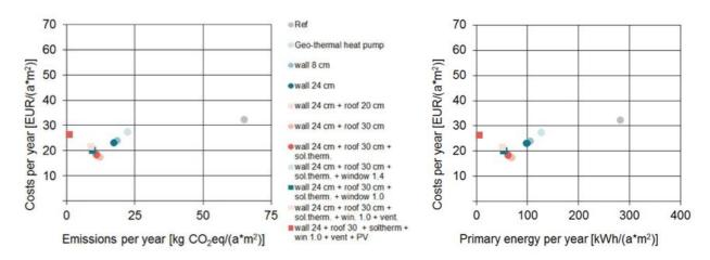
Figure 9: Comparison of cost effectiveness of energy efficiency renovation measures for the Austrian Case Study for a geo-thermal heat pump system, as well as related impacts on carbon emissions and primary energy use
