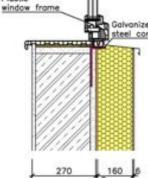
Figure 12: Cross section of the exterior wall and window. Window frame installed on galvanized steel consoles (red) protructing to new EPS thermal insulation layer (beige).
