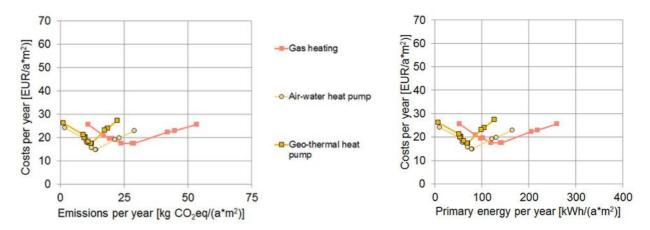
Figure 11: Aggregated comparison of cost effectiveness of energy efficiency renovation measures for different heating systems and related impacts on carbon emissions and primary energy use for the Austrian Case Study (part II)
