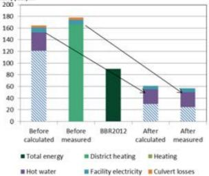
Figure 14: The energy use before and after renovation. BBR2012 is the building code requirement for new construction.
