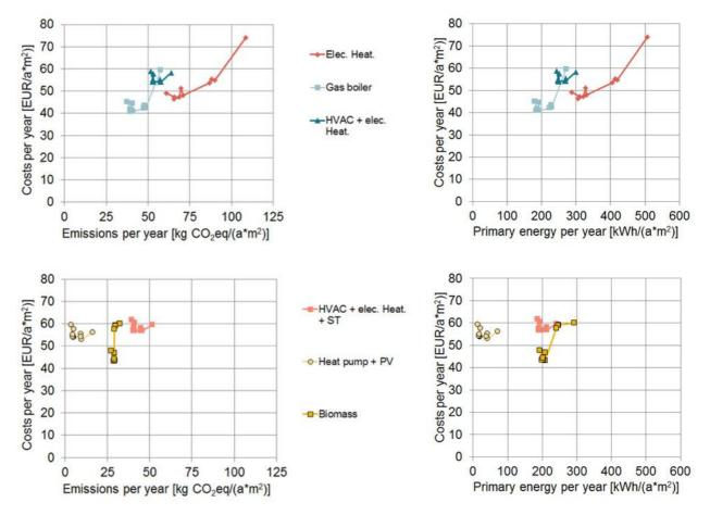
Figure 20: Aggregated comparison of cost effectiveness of energy efficiency renovation measures for different BITS and related impacts on carbon emissions and primary energy use for the Portuguese Case Study
