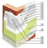
Figure 24: Exterior thermal composite system insulation.
