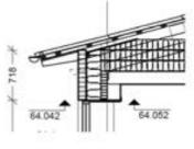
Figure 15: Section showing added roof insulation - new total: 435 mm
