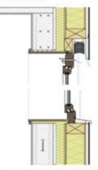
Figure 14: construction detail of the window incl. shading device
