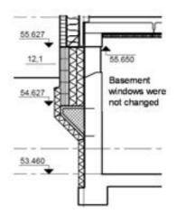
Figure 10: The external insulation is continued to the base of the building to reduce/avoid thermal bridges
