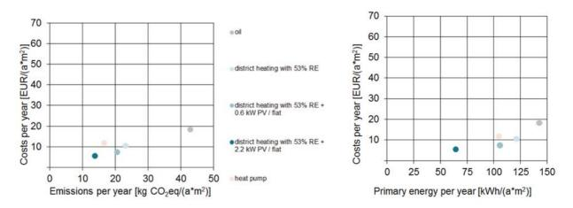
Figure 14: Comparison of cost effectiveness of energy efficiency renovation measures for the Danish Case Study for the different heating systems, including renewable energy generation on-site by the photovoltaic installation, only reference case
