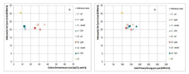
Figure 6: Life Cycle Costs in comparison with carbon emissions (left chart) and total Primary Energy (right chart) of the Case Study "Kapfenberg", Austria
