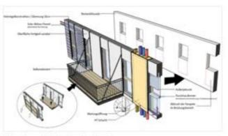
Figure 8: prefabricated façade element
