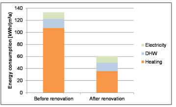
Figure 23: Differences in energy consumption before and after renovation.
