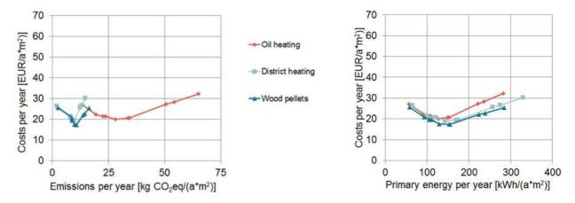
Figure 10: Aggregated comparison of cost effectiveness of energy efficiency renovation measures for different heating systems and related impacts on carbon emissions and primary energy use for the Austrian Case Study (part I)
