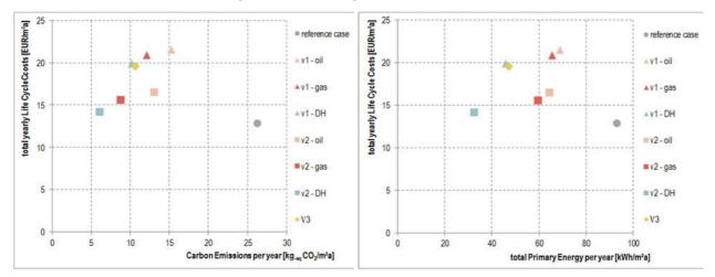
Figure 12: Life Cycle Costs in comparison with carbon emissions (left chart) and total Primary Energy (right chart) of the Case Study "Traneparken", Denmark
