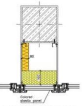
Figure 15: Detail of installation of plastic panel in front of the load/bearing reinforced concrete column. EPS thermal insulation (beige) is installed from the interior side. Acoustic insulation made of mineral wool (orange) is also visible.
