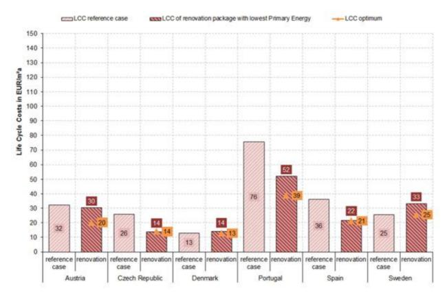
Figure 41: Life Cycle Costs of the six Case Studies. The LCC of the reference cases are compared to the LCC of the renovation packages, which achieve the lowest total Primary Energy. Additionally the LCC optimum for each Case Study was marked.
