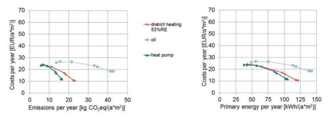
Figure 15: Aggregated comparison of cost effectiveness of energy efficiency renovation measures for different heating systems and related impacts on carbon emissions and primary energy use for the Danish Case Study
