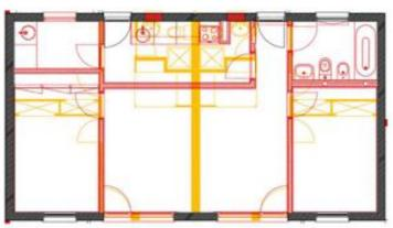
Figure 5: Renovation plans (in yellow demolitions and in red new elements)
