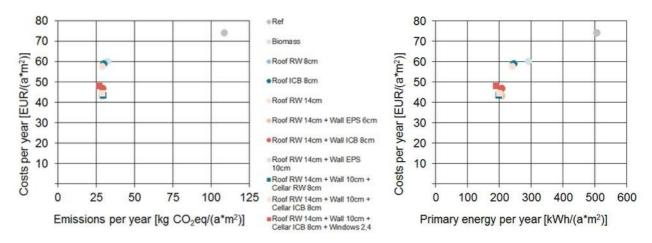
Figure 19: Comparison of cost effectiveness of energy efficiency renovation measures for the Portuguese Case Study for a biomass system, as well as related impacts on carbon emissions and primary energy use
