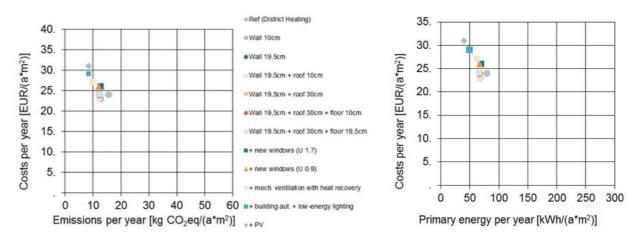
Figure 27: Comparison of cost effectiveness of energy efficiency renovation measures for the Swedish Case Study for district heating (partly based on renewable energy sources), as well as related impacts on carbon emissions and primary energy use.
