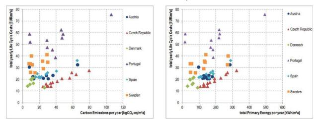
Figure 43: Comparison of Life Cycle Costs, carbon emissions (left side) and total Primary Energy (right side) of all investigated Case Studies
