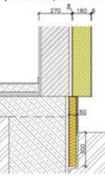
Figure 7: Base of the exterior wall after renovation. Added EPS thermal insulation (beige) is covered by acrylic plaster. The plinth is insulated by XPS (orange), covered by ceramic tites.
