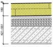
Figure 10: Renovation of the roof. Additional EPS thermal insulation (beige) and modified (SBS) bituminous sheets (black) with mineral granules.
