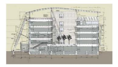
The ventilation rate by natural ventilation is estimated with ventilation network calculation. When there is 1.0 m/s external wind, the ventilation rate in major rooms in Itoman city hall
