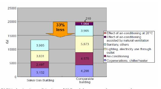
PMV index in air-conditioning at 28°C and the amount of energy saved
