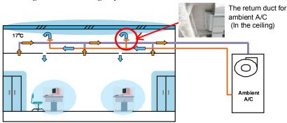
In summer, by keeping the climate control system operating at night, cold is stored in the flooring slabs, furniture and interior materials. Then this cold is released during the day-time, and we can reduce energy consumption during the peak electricity usage period by approximately 20%.
