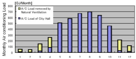
Estimated AC load removed by natural ventilation.
