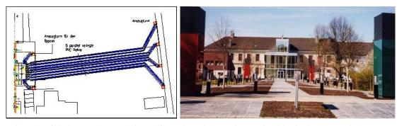
Schematic of the heat exchanger (left) and front view of the conference facilities flanked by two inlet towers.
