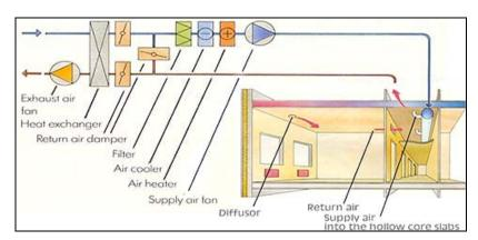
TermoDeck schematic diagram. Source: http://www.termodeck.com
