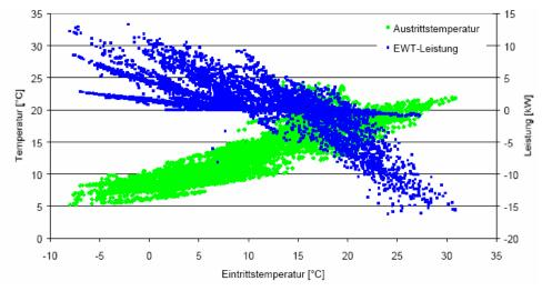
The underground heat exchanger performance and the outlet temperatures as a function of the inlet temperature. (*Eintrittstemperatur* = inlet temperature and Leistung = yield of the underground heat exchanger).
