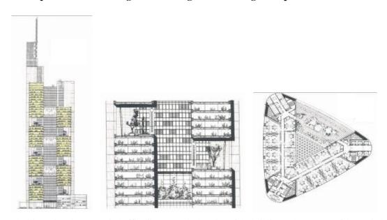
The illustration shows a typical office floor, a vertical section of the building and a segment of the vertical section. This gives an idea of how the atrium and the winter-gardens are placed in the building. The atrium is placed as a vertical core in the centre of the building, connecting the four storey winter-gardens and ensuring ventilation. Need permission
