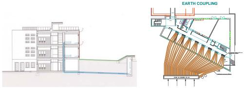
Earth coupling system and cooled air supply.
