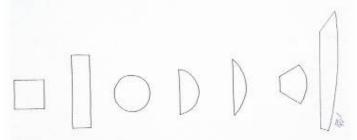
The illustration shows the shapes investigated in relation to the volume to surface ratio. The five on the left side are the investigated shapes and the one on the right is the final shape. Need permission
