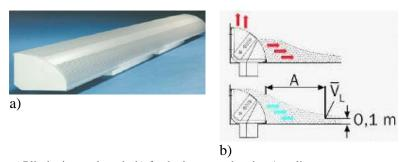
a) Plinth air supply unit, b) fresh air pattern heating / cooling
