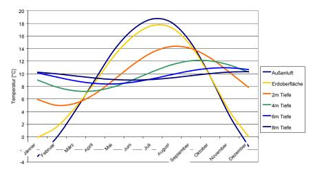
Annual temperature of outdoor air, surface of the earth and earth at different depths for the soil types "pebble stones –dry", location Graz. The graph is based on the mean monthly values.
