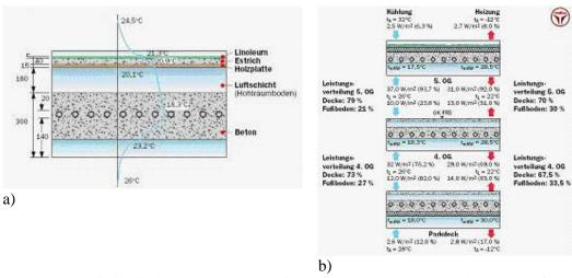
a) Temperature distribution in the concrete slab during the cooling mode; b) Thermal output rates from the activated slab for different floors of the building
