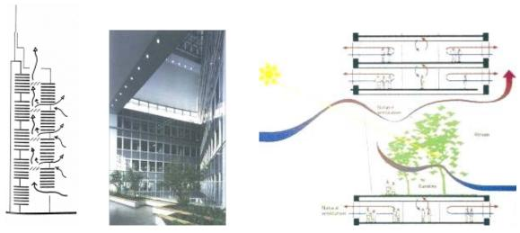
The atrium works as a chimney for the ventilation air. The winter-gardens also work as a thermal buffer during the winter and summer season. In winter it is used to preheat the natural ventilation, while in summer it is used to cool down the external air by 0.5 and 1°C through evaporative cooling. Need permission
