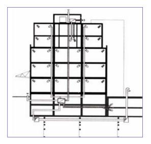
Figure 3-33 Schematic of Schwerzenbacherhof building ventilation system
