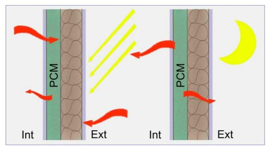
Figure 3-38 Scheme of PCM application on the inner side of the wall
