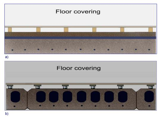
Figure 3-21 Basic types of currently used water based thermo active building components: a) on-site constructed floor (with insulation); b) hollow deck with integrated pipes
