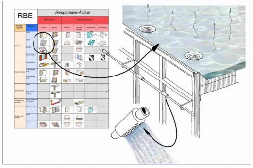
Figure 3-55 Activating the water layer on a roof.
