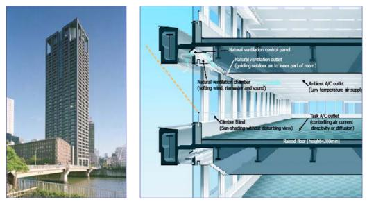
Figure 3-27 Existing application of ACSuBTS - KANDEN Building of Kansai Electric Power Company, Inc. (KEPO) in Osaka, Japan
