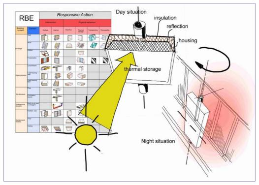
Figure 3-54 Activating the thermal mass in combination with ventilation.
