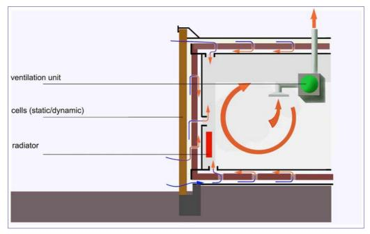
Figure 3-50 DI concept and working principle
