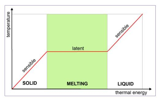
Figure 3-36 Specific thermal energy (stored) vs. temperature
