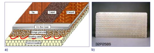
Figure 3-41 A typical configuration of a floor heating system coupled with PCM b) Example of a PCM container for floor
