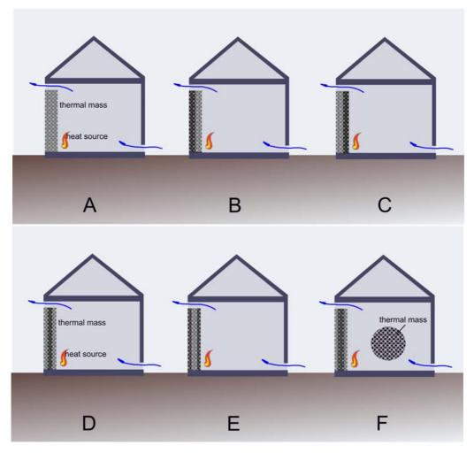
Figure 3-17 Illustration of six simple building models with different relative location of the thermal mass to the insulation and the existence of internal thermal mass
