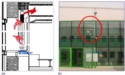
Figure 3-13 Environment Park in Turin, Italy a) The monitored climate facade b) Scheme of the working principle of the facade
