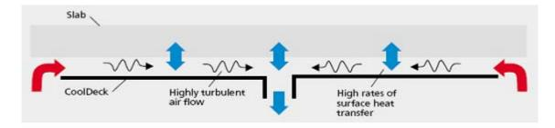
Figure 3-49 Stevenage Borough Council" building - Scheme of the working principle of the PCM based ceiling
