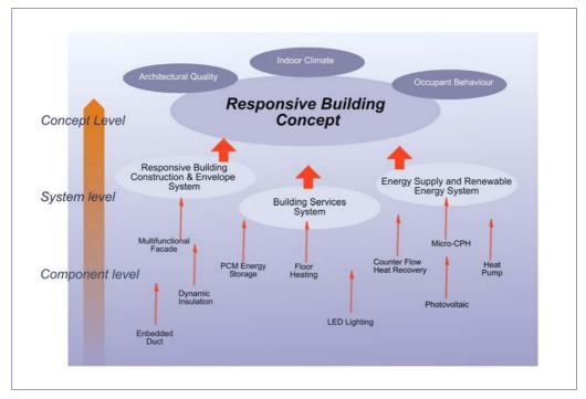
Figure 1-2 Illustration of the Responsive Building Concept
