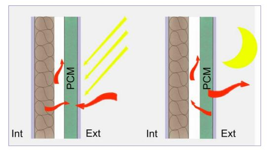
Figure 3-40 Scheme of the application of PCM in a solar wall
