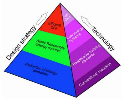
Figure 4-4 Illustration of Annex 44 Design Strategy and corresponding technologies. CFF: Clean fossil fuels.
