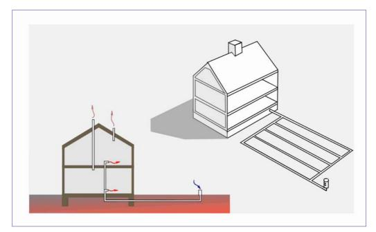
Figure 3-30 Building with an Earth-to-Air Heat Exchanger
