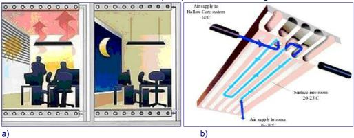
Figure 3-18 Thermal mass activation working principles a) SA activation involves only the surface of the element b) CA activation involves the whole structure (core) of the element.
