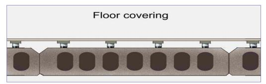
Figure 3-20 Principle of a hollow deck with cavities for air circulation
