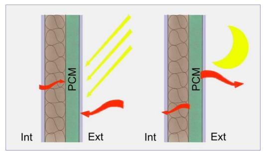
Figure 3-39 Scheme of the application of PCM on the external side of the wall
