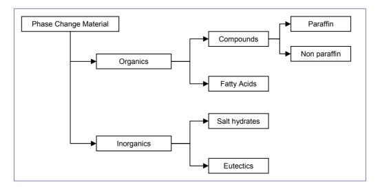
Figure 3-37 Different typologies of Phase Change Materials
