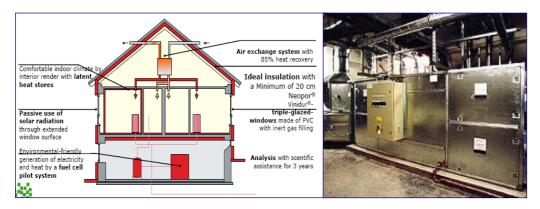
Figure 3-45 Schematic cross-sections and air handling and heat recovery "3-litre house"
