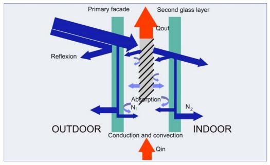
Figure 3-3 DSF/AIF working principles
