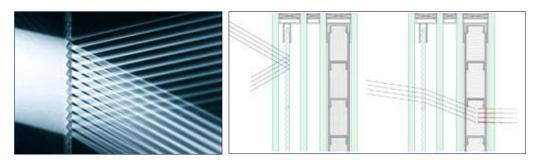
Figure 3-47 Domat Ems building - Particular of the south facing solar wall
