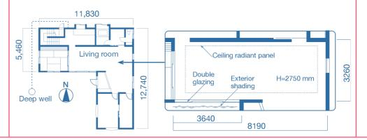
Figure 20. The house equipped with ceiling radiant cooling system using well water (Asada and Takeda 2002).
