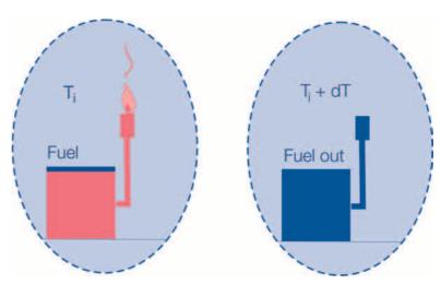
Figure 7. Combustion of fuel in air as an example to show the difference between energy and exergy analysis (Moran 1989, modified).
