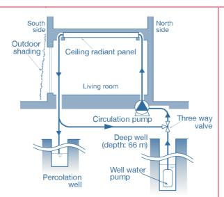
Figure 21. Components and well water flow (Asada and Takeda 2002).
