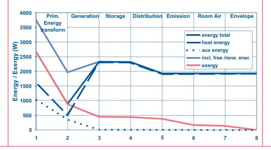
Figure 22. Exergy analysis of a floor heating system using a heat pump as energy generator.
