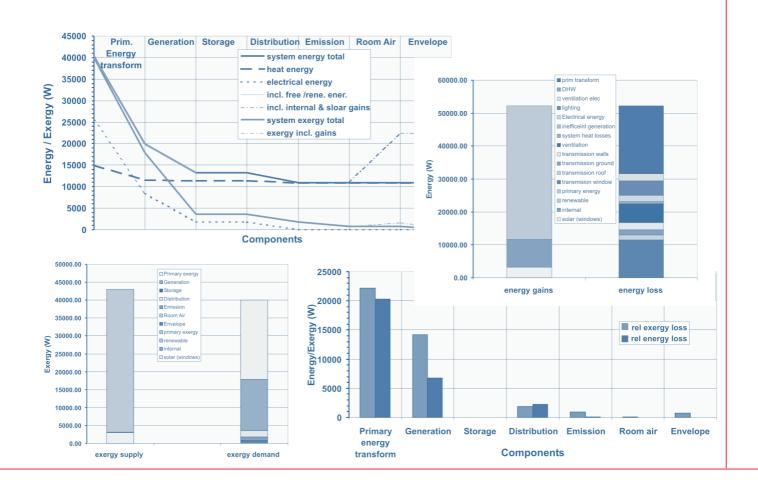
The objective of the "Pre-Design Tool for Energy and Exergy Analyses of Heating and Cooling Applications in Buildings" is to provide designers or users with a simple tool that shows a holistic image of the energetic-flow and exergetic-flow patterns of various low temperature heating and high temperature cooling systems in buildings. For this purpose, the tool includes a program that estimates the heating and cooling requirements of a building using the well-known modified-bin
