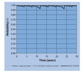
quality and the load on the system. Figure 20 and Figure 21 show the reliability of a mechanical ventilation system with heat recovery and an average quality level with a normal maintenance level and a poor maintenance level respectively. Reliability is expressed as a fraction between 0 and 1, meaning the probability that a system can fulfil the specified requirements between certain time intervals. Reliability means:
