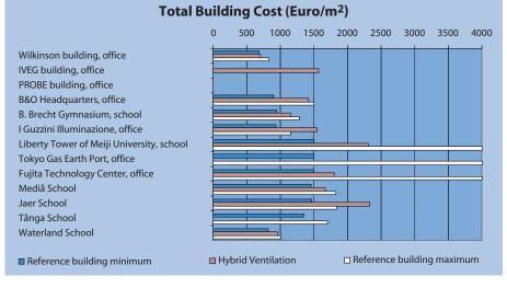
case study buildings indicate a potential for cost savings, especially with regard to installation costs. The installation cost in hybrid ventilated buildings is approximately 20-25% of the total building cost.
