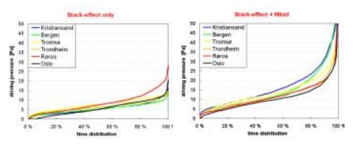
Figure 2a: Prevalent stack-effect driving forces.
