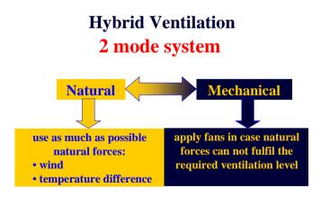
Figure 2: Schematic picture of hybrid ventilation.
