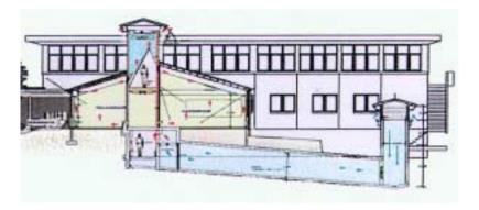
*Figure 6: Gronge school Norway a typical example of a hybrid ventilation system.*
