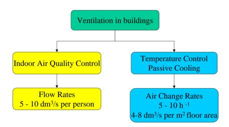
*Figure 3: Functions of a ventilation system.*
