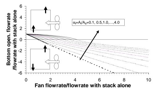
*Figure 4: Flow rate through the bottom opening in a two-opening mixed-mode building with stack driven ventilation and a supply fan.*
