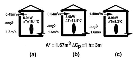
Figure 3: Three flow states in a building with identical ventilation parameters. The downward flow of  $0.54 \text{ m}^3$ /s is not stable, as shown by Li and Delsante (2000).
