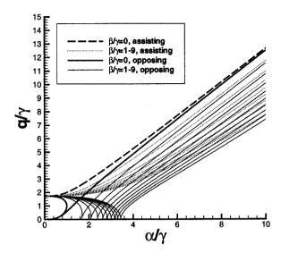
Figure 2: Ventilation flow rates for combined forces – both opposing and assisting winds. Where q is the ventilation flow rate,  $\alpha$ ,  $\beta$  and  $\gamma$  are the thermal buoyancy-, envelope heat loss- and wind- air change parameters, respectively. For a certain range of  $\alpha/\gamma$ , there are two stable solutions and one unstable solution.
