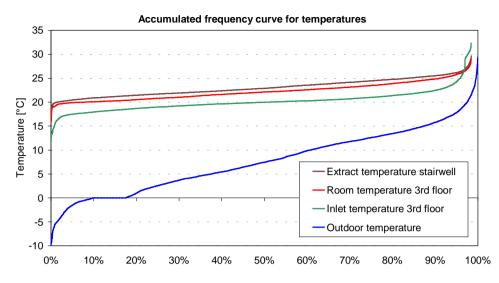
*Figure 4:* Average temperature levels at third floor. Temperature data are logged by the BEMS system from each temperature sensor. Average values are shown for the third floor.
