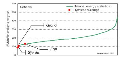
*Figure 6:* Distribution of specific energy consumption (not degree-day corrected) in kWh/m<sup>2</sup> heated area from the national database of energy consumption in 356 school buildings [7]. Three HybVent buildings are plotted as red dots.
