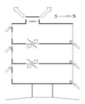
Figure 2: Principle of hybrid ventilation system (Aggerholm, 1999).
