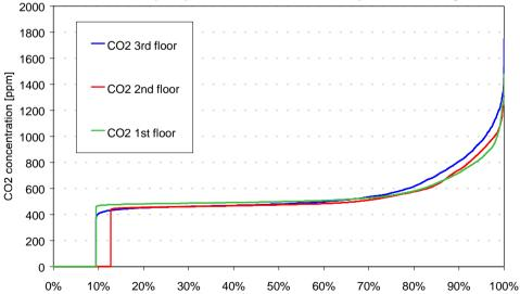
Figure 3: CO<sub>2</sub> levels at each office floor based on one year of monitoring. CO<sub>2</sub> concentrations are logged by the BEMS system.
