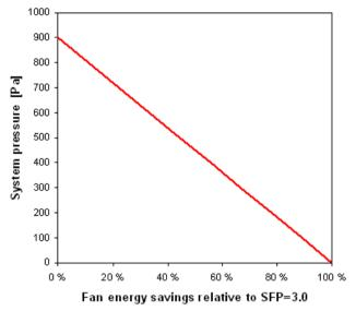
*Figure 3:* Fan energy savings for different system pressure losses, relative to a system with SFP=3.0.
