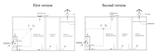
Figure 2. Scheme of ventilation system of Waterland school building.
