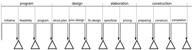
Figure 4: The design process subdivided into four stages and eleven phases<sup>1</sup>
