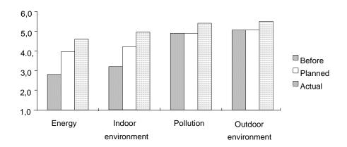
The Ecoprofile shows significant environmental improvements both from the nonrenovation phase to the planned phase, and even improvements from the planned phase to the actual building. The improvements are especially within energy and the indoor environment.
