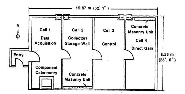
Fig. 14. Floor plan of the NBS passive solar test building
