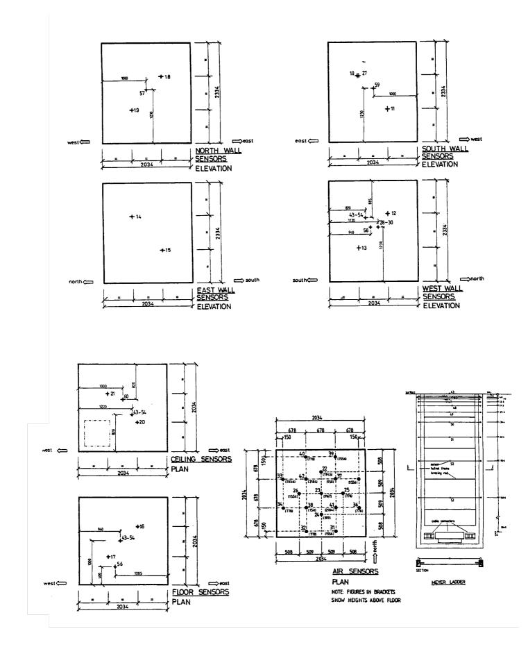
Fig. 6. Sensor locations in the British Gas test cell during the winter of 1990
