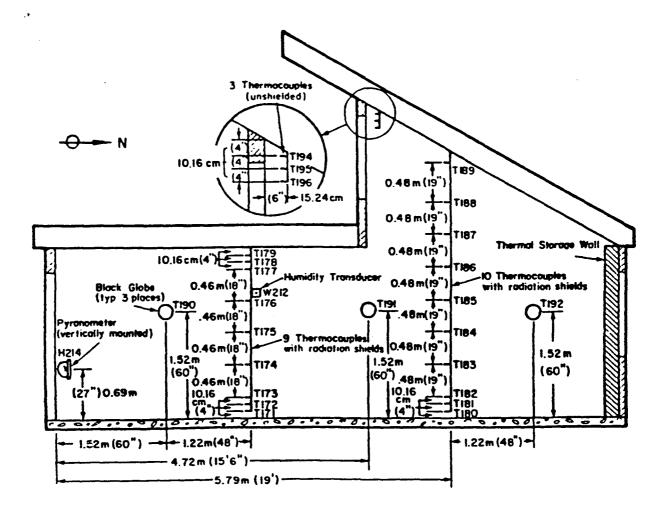
Fig. 15. Longitudinal section and air temperature sensors in the IEA Solar Heatng and Cooling Program direct gain cell 4 Task 12
