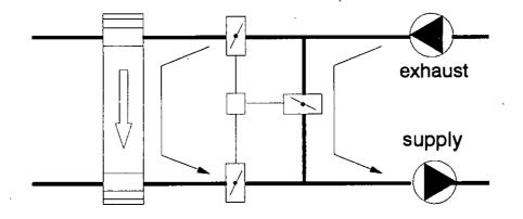
Figure 9.5. Configurations that will result in short circuiting.
