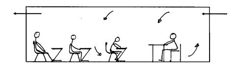
Figure 8.7. Principle function of a ventilating system with mixing devices.
