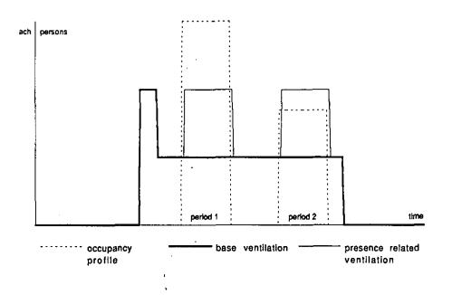
Figure 5.8. Adaptation of ventilation rate according to the presence
