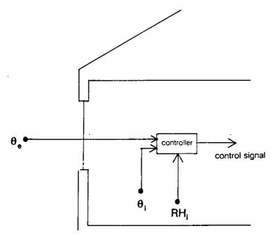
If the surface temperature  $\theta_s$  can not be directly measured, it can be calculated if the temperature ratio at the critical spot is know; however, the extension temperature has to be measured.
