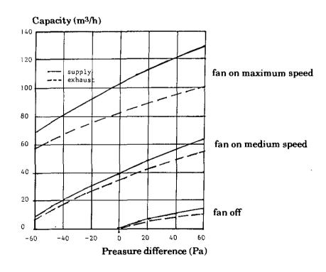
Figure 7.8. Influence of pressure difference on flow rate from wall mounted fans
