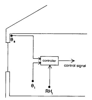
The surface temperature is directly measured at the critical/coldest spot of the wall (see [4]).
