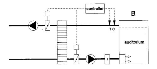
Figure 9.3. DCV system with throttling dampers.
