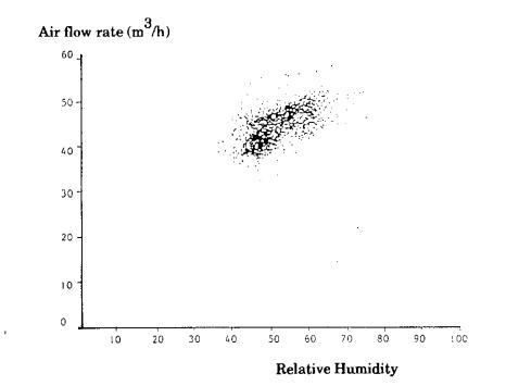
Figure 7.5. The air flow rate for a system governed by a RH-sensor, demonstration project Orsay, France.
