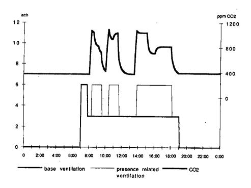
Figure 5.10. Ventilation operation with two-speed fan
