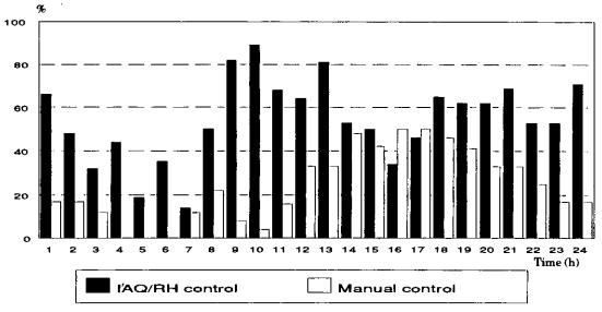
Figure 7.12. Percentage of time of fan operation at high speed as a function of time of the day
