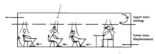
Figure 8.6. Principle function of a ventilating system with displacement devices
