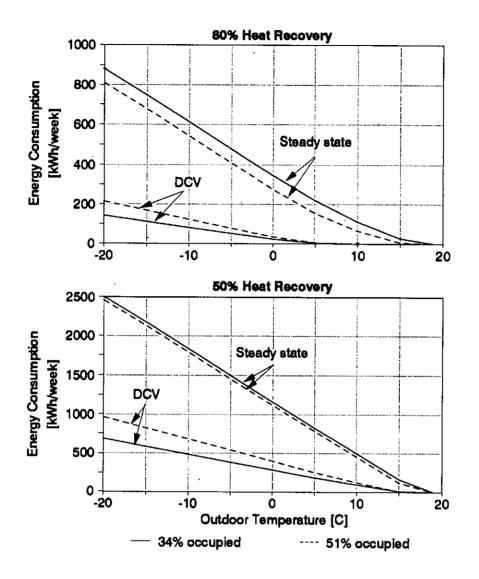
Figure 9.6. Energy consumption as a function of heat exchanger efficiency, outdoor temperature and occupancy.
