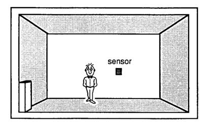
Figure 5.12. Location of sensor in the occupied zone
