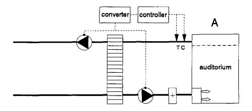
Figure 9.2. DCV system with variable speed-controlled fans.
