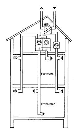
b Two zone air heating system with outdoor air to the bedrooms and recirculation air to the hvingroom
