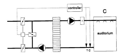
Figure 9.4. DCV system with return air
