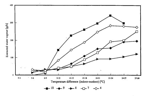
Fig. 6: calculated average values for extracted quantities of water vapour, Schiedam, reference apartments(wind speed 0-2 m/s).
