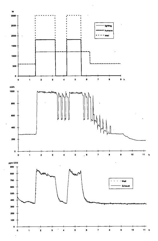
Figure 1; Load, air flow rate and  $CO_2$ -concentration during test No 11.
