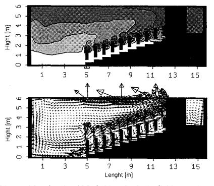
Fig. 11. Mass fraction  $(CO_2/Air)$  and velocity field at section yz19.
