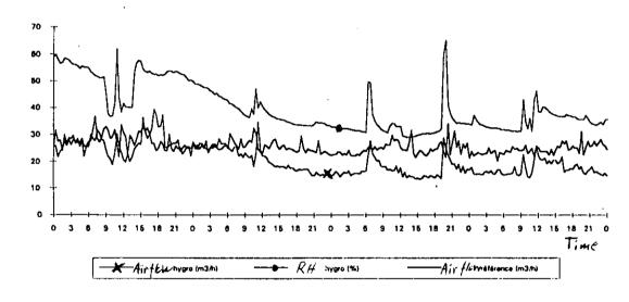
Fig. 8: air flow rates in a similar reference and humidity controlled apartment as well as the relative humidity in the humidity controlled apartment, Les Ulis, January 1990[1]
