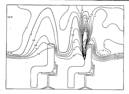
Figure 4 Iso-concentration map showing the dispersion pattern of a tracer gas emitted close to one of the two heated dummies. Concentrations are given relative to that in the extract
