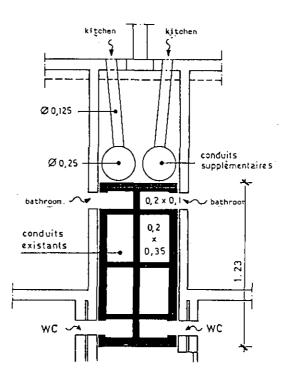
Fig. 4 : Sections of ventilation ducts in Namur building
