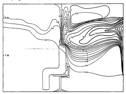
Figure 6 Iso-concentration map showing the dispersion pattern of a tracer emitted close to the wall in the lower zone. One heated dummy is present. Concentrations are given relative to that in the extract.
