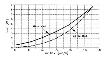
Fig. 6. Relationship between fan speed and electric load.
