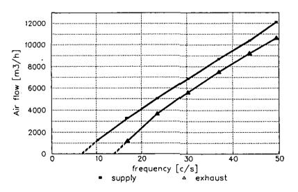
Fig. 5. Air flow rate as a function frequency output.
