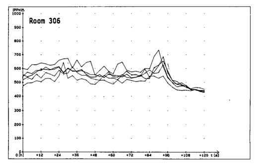
Fig 10. CO2-concentration in 6 points at 0.1 m level
