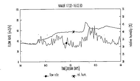
Fig. 5 : example of the measured variables (reference apartment)
