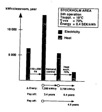
As shown in Fig. 11, increasing the fresh air flow specified in the existing building code (5 l/s per student, 150 l per class) to a fresh air floor guaranteeing good air quality – for example, a maximum of 800 ppm of  $CO_2$  (10 l/s per student, 300 l per class), doubles the energy requirement for air handling.
