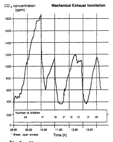
Fig 2. CO<sub>2</sub>-concentration in a classroom before renovation
