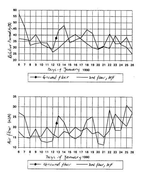
Fig. 9 : daily average air flow rates and relative humidity levels in 2 humidity controlled apartments Les Ulis, 6 to 26 January 1990[1]
