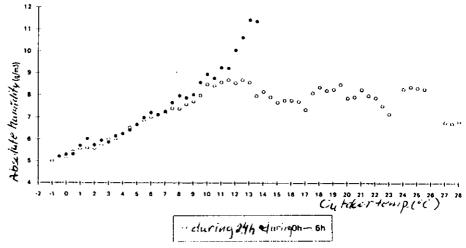
Fig. 7: Measured average absolute humidity as a function of the outside temperature during the monitoring campaigns in Les Ulis[1]
