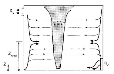
Figure 1 Principle of ventilation by displacement
