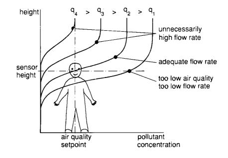
Figure 2 Principles for demand control of ventilation rate in a room ventilated by displacement.
