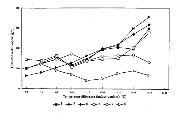
Fig. 7: daily extracted water vapour quantities as function of temperature difference. (wind speed 0-2 m/s)
