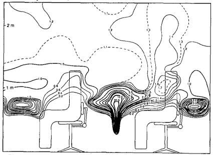
Figure 5 Iso-concentration map showing the dispersion pattern of a tracer gas emitted directly above a 4 W heat source in the lower zone. Concentrations are given relative to that in the extract.
