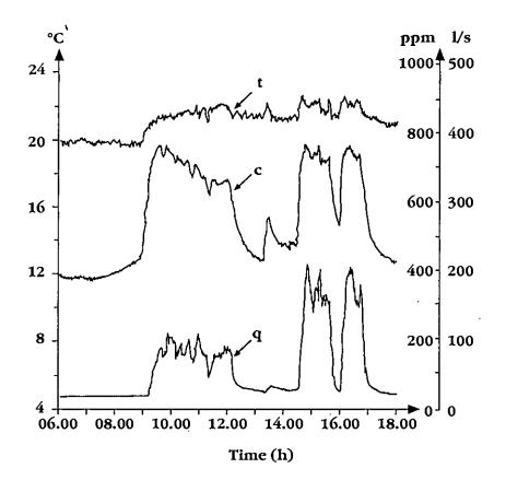
Figure 3. Measured values of room temperature (t), carbon dioxide concentration (c) and supply air flow (q) in the conference room for a working day during which the occupant load varied widely.
