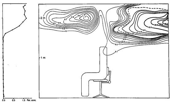
Figure 7 Iso-concentration map showing the dispersion pattern of a tracer gas emitted close to the wall in the upper zone. Concentrations are given relative to that in the extract. Also shown (to the right) is the vertical concentration profile of a tracer released close to the ceiling.
