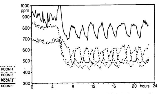
Figure 3 Concentration histories at 1.2 m height in the four rooms, when room 1 is the source room with three simulated persons. The total flow rate is 120 m<sup>2</sup>/h during the first 5 hours, thereafter 240 m<sup>2</sup>/h. The doors are open
