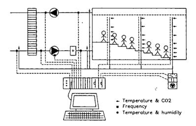
Fig. 4. Data acquisition system and sensor arrangement.
