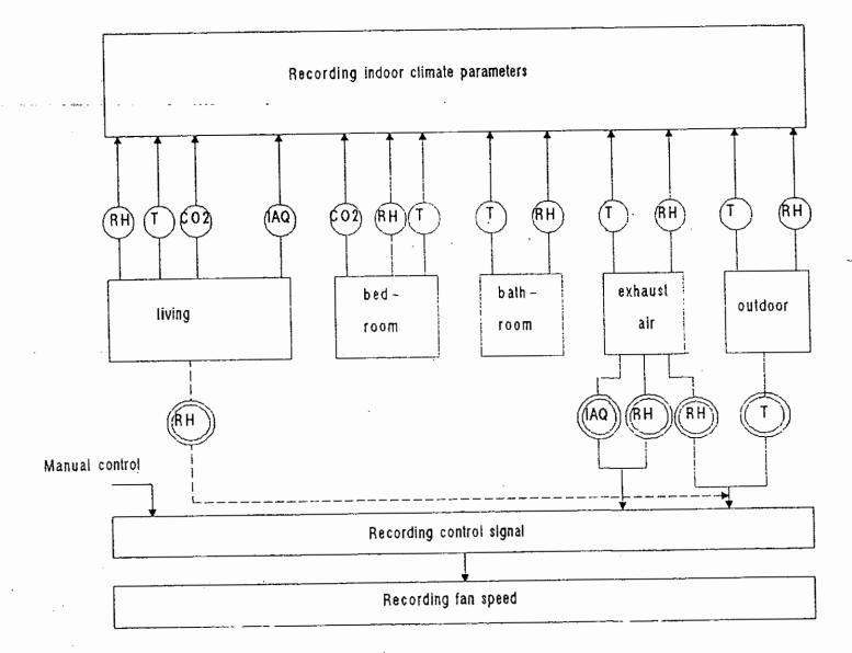
Figure 4. Monitoring scheme of the measuring set up.
