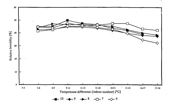
Fig. 5: variation of the average relative humidity as function of the temperature difference between inside and outside, Schiedam, reference apartments (wind speed 0-2 m/s)
