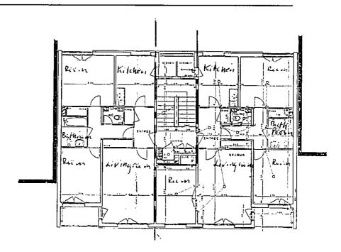
Figure 2: Ground plan of one of the reference apartments in the Ulis building
