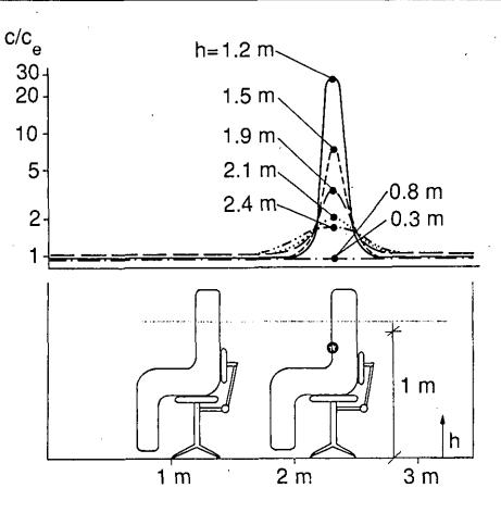
Figure 8 Mixing ventilation. Concentration profiles at different heights above the floor. The tracer gas source is positioned close to the heated body at 0.85 m height.
