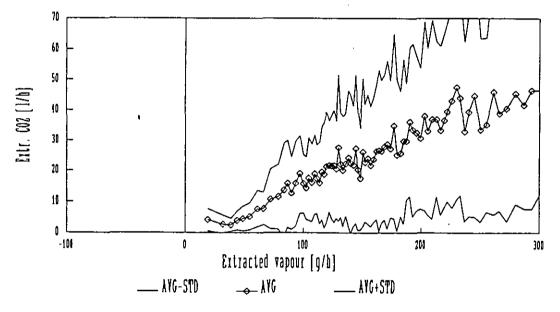
Fig. 11: relation between extracted water vapour and  $CO_2$ -rates, Namur, reference apartment 6, bathroom, whole period.
