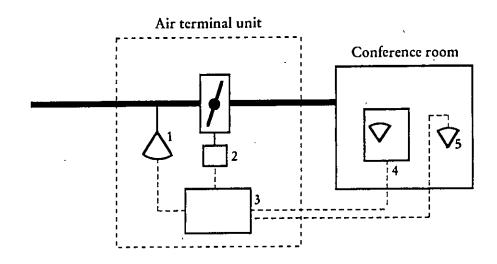
Figure 2. Diagrammatic arrangement of the control system for the conference room: 1) air flow sensor, 2) damper, 3) control unit, 4) room temperature sensor and set point selector, 5) carbon dioxide sensor.
