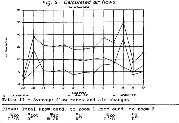
The total average ach's was close to 0.50, while the peak number of ach's was 0.83, indicating an air flow reduction of 40 , whether a constant ventilation system would have been adopted.
