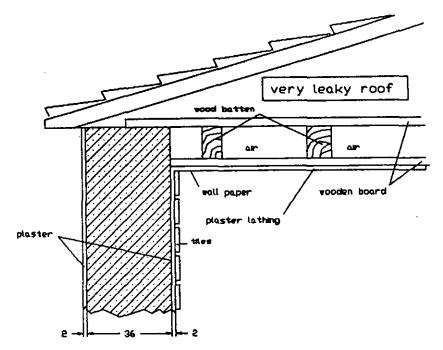
Figure 7: Schematic of the wall and roof design of the bathroom
