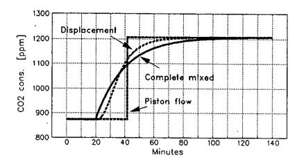
Fig. 13. Process response as a function of air flow pattern
