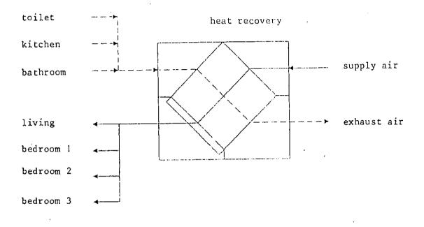
Figure 2. Principle scheme of the balanced ventilation system with heat recovery.
