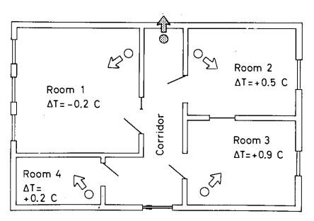
Figure 1. Plan of the test building. The south wall is an external wall of the laboratory hall, while all other walls are inside the laboratory hall. The  $\Delta$ T-figures denote the difference between the mean room temperature and the temperature in the corridor when the room is a source room
