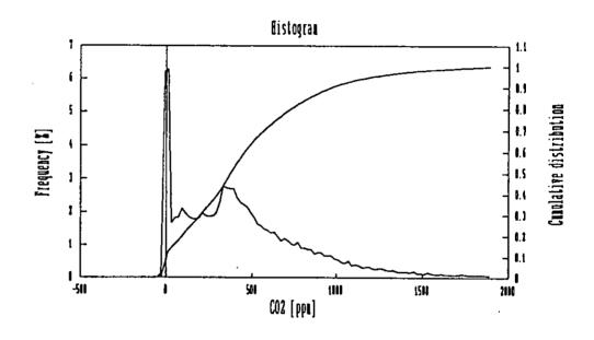
Fig. 9: histogram of measured CO<sub>2</sub>-concentrations and cumulative histogram, Namur building, reference apartments (difference hetween iodoor and outdoor)
