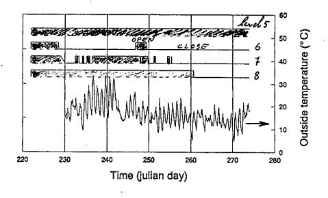
Fig. 12: use of ventilation grills in reference apartments in Namur building (Augustus-September 1990, floor 5 to 8)
