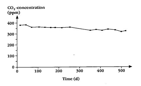
Figure 4. Background carbon dioxide concentrations, according to measurements with the sensor used for control of the supply air flow to the conference room. The values given are average values for an 8 hour period during Sunday mornings when the room was unoccupied.
