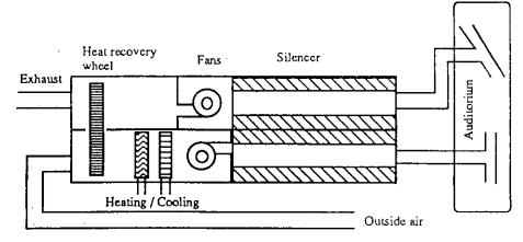
Figure 3: System sketch of the ventilating system
