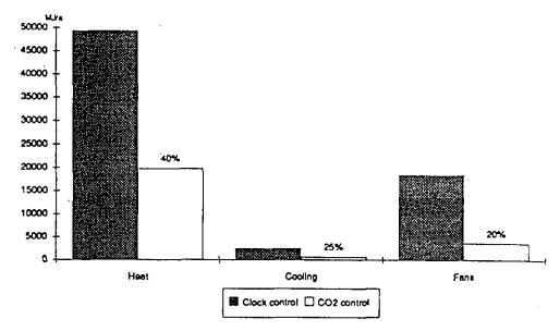
Figure 7: Calculated energy consumption for monitored operating conditions
