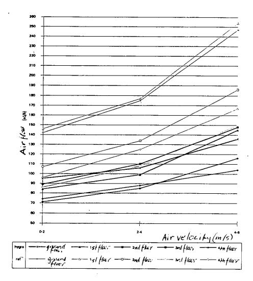
Fig. 11: variation of the average air flow rates as function of the wind velocity, outside temperature between 4 and 7 °C,Les Ulis [1]
