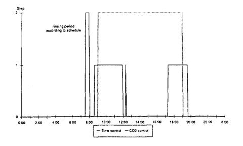
Figure 5: Operation of the ventilating system with clock control and CO<sub>2</sub> control. (same weekday; occupancy: 15 - 20 persons) Even in summer the room air temperature never rose above the threshold value of 27 °C, which means that in practice the operation of the ventilating system was only controlled by the CO<sub>2</sub>-sensor.
