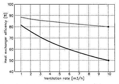
Fig. 7. Relation between the heat exchanger efficiency and the air flow.
