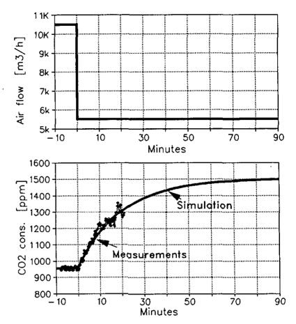
Fig. 12. Step response in the exhaust duct (measurements and computer simulations)
