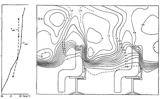
Figure 3 Iso-concentration map showing the dispersion pattern of a tracer gas emitted close to the ceiling. The concentration figures are given relative to the concentration in the extract. The dummies are situated in the measuring plane and are heated with 100 W power. Also shown are the vertical temperature profiles at the wall and in the room air.
