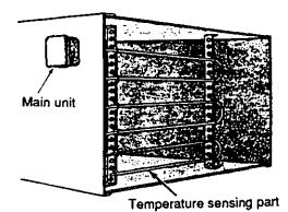
Fig. 4.11 An example of Average Temperature Measurement <sup>JN 12</sup>
