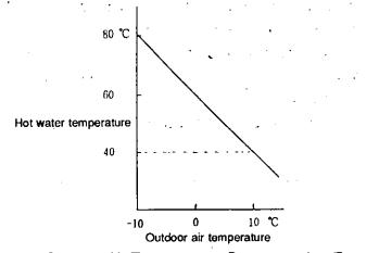
Fig. 9.2 Outdoor Air Temperature Compensation Example
