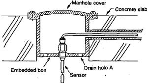
Fig. 4.9 A Mounting Example Inside a Manhole
