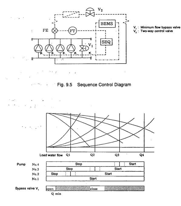
Fig. 9.6 Pump Characteristics and Sequence Control
