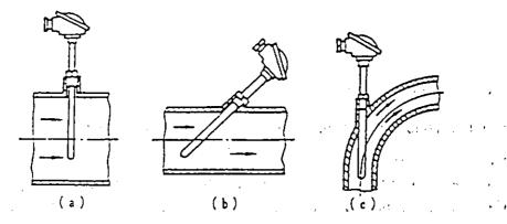
Fig. 4.12 An Installation Example of a Resistance Thermometer Bulb to Piping <sup>JN 3</sup>
