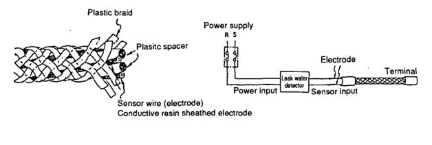
Fig. 5.2 An Example of Sensor Cables
