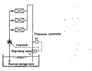
Fig. 4.14 Return Water Pressure Control JN 20)
