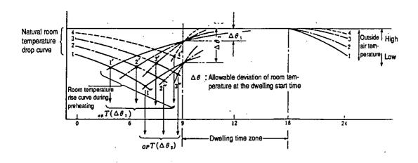
$_{op}T(\Delta\theta)$ : Optimal start-stop time when allowable deviation of room temperature is  $\Delta\theta$ .
