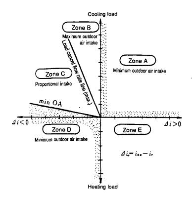
Fig. 4.7 Outdoor Air Intake Strategy in Airconditioning JN 2)
