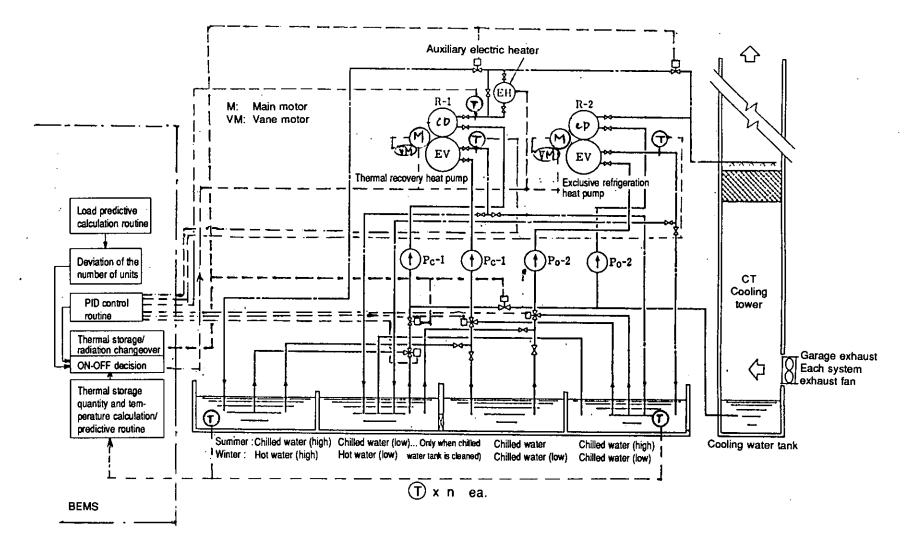
Fig. 9.12 Heat Pump Sequence Control Block Diagram
