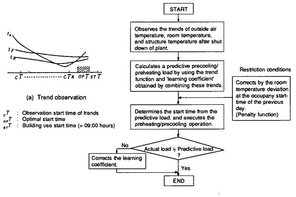
(b) Outlined optimization flow of preheating/precooling operation
