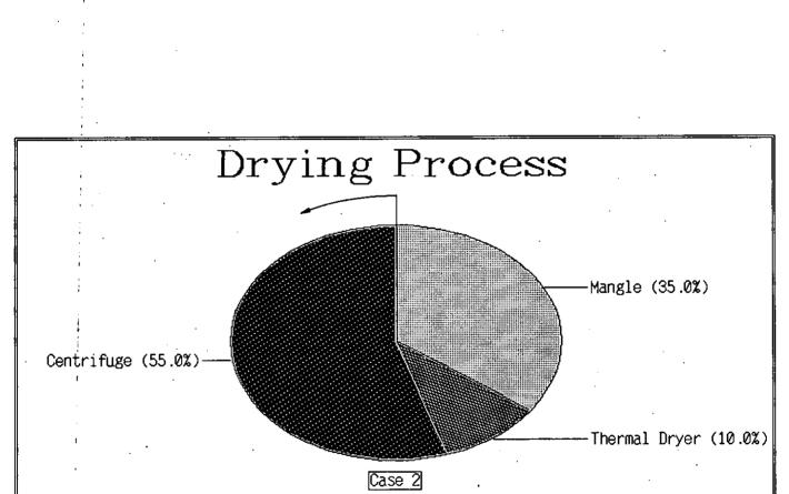
Fig. 2.2.A. - Percentage of water removed in each step of a 3 phase process
