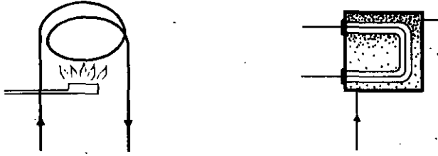
Fig. IV b-4 Individual appliances for hot water generation without accumulation. Gas (left) and electric (right)
