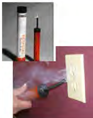
Smoke Pencil or similar tool to Provide show of air flow
