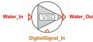
Fig. 7.28: Connector types in Simergy shown on a pump (graphical representation)
