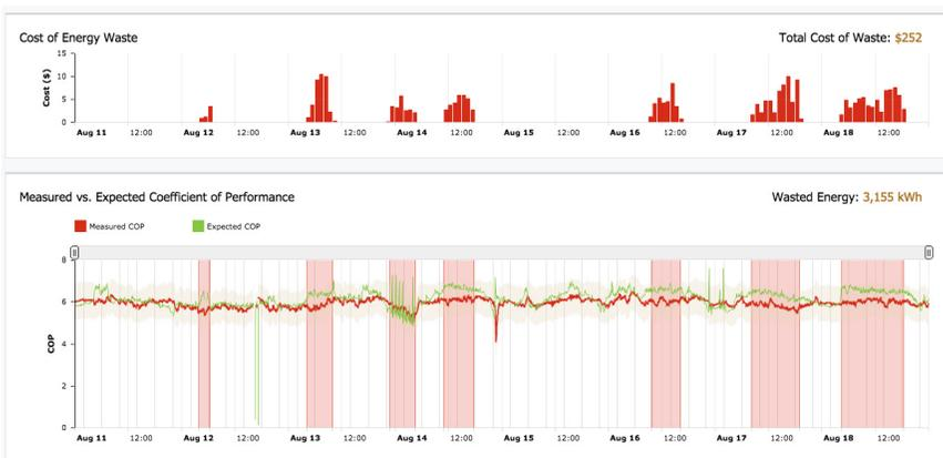
Fig. 11.5: Outputs of the fault identification algorithm, with costs caused by the fault (top graph) and comparison between measured and expected COP (bottom graph). The red rectangles are time intervals that have been identified as faulty periods in which the performance of the chiller was outside the tolerance.
