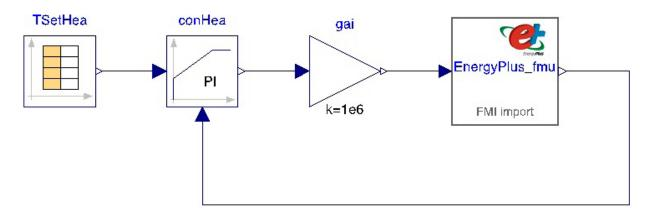
Figure 3: Modelica system model that connect a feedback controller with an EnergyPlus whole building model, which has been exported as an FMU.
