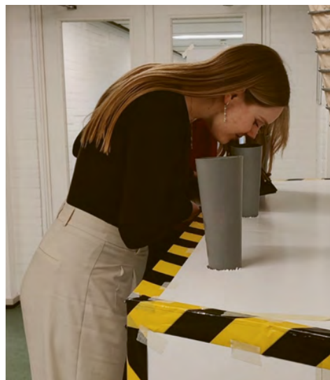
Testing of perceived air quality with whole body exposure (left) and use of funnels (right). Source: International Centre for Indoor Environment and Energy, Technical University of Denmark
