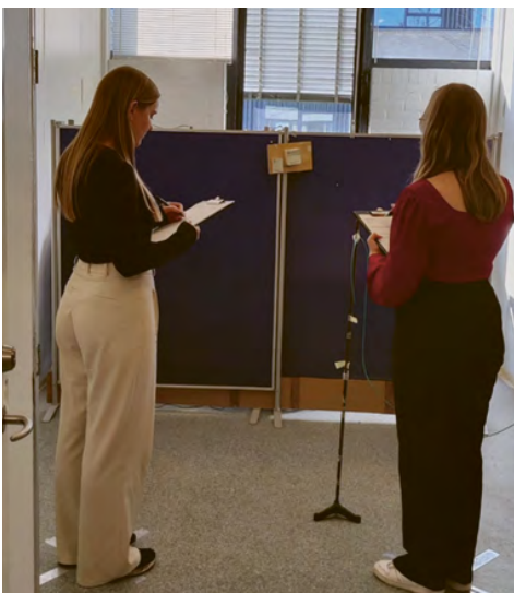
Testing of perceived air quality with whole body exposure (left) and use of funnels (right). Source: International Centre for Indoor Environment and Energy, Technical University of Denmark
