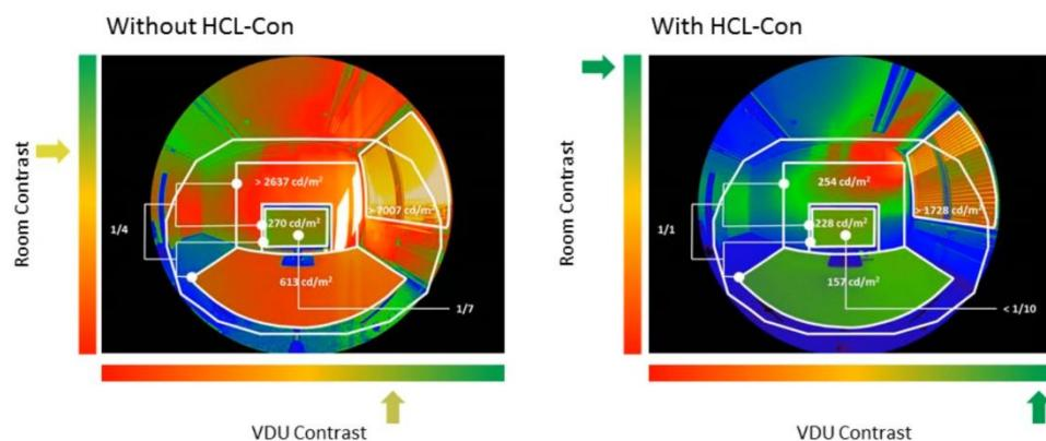
*Lighting scenes with the same basic parameters were compared in pairs of images, each with conventional (inadequate) lighting control and with optimised HCL-Con lighting control. © Fraunhofer IBP*
