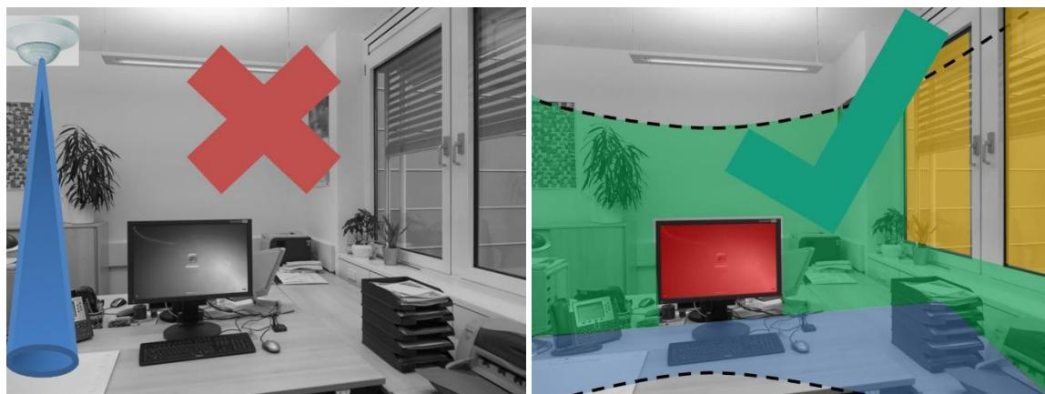
*Conventional lighting controls detect and regulate horizontal illuminance levels (left), but the user comfort is predominantly in the vertical field of vision (right). © Fraunhofer IBP*
