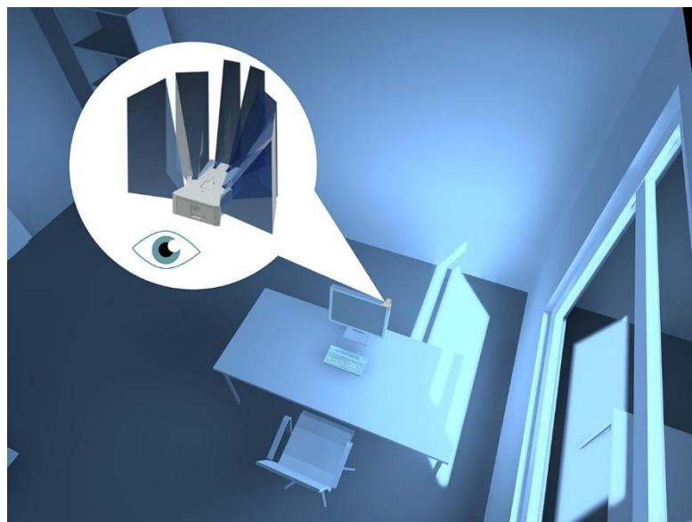
*Concept of the HCL-Con sensor for the detection of vertical illuminance levels. © Fraunhofer IBP*
