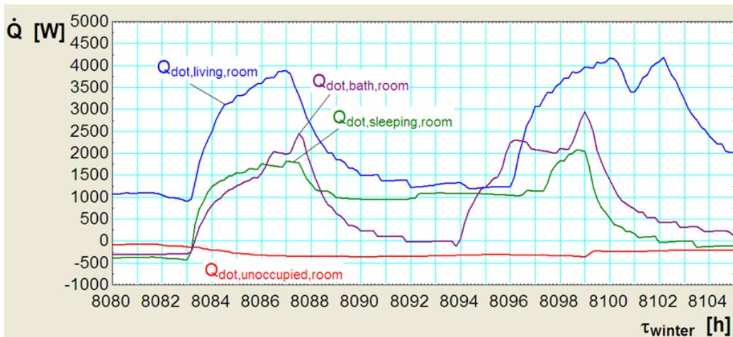
Figure 7-25: Simulated heating demands as functions of the four indoor temperatures of Figure 7-23
