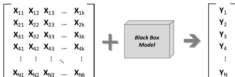
Figure 7-3: Scheme of sampled inputs matrix and model outputs vector.
