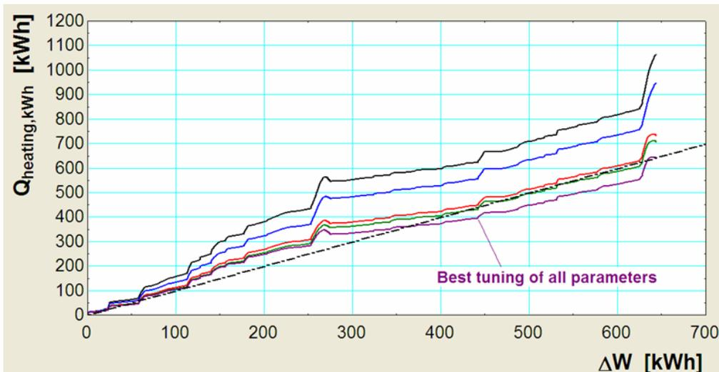
Figure 7-31: Simulated heating demand as function of the electricity consumption
