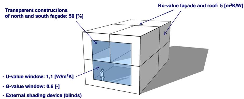
Figure 4-4: Shoe-box design used in the Netherlands
