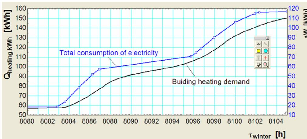
Figure 7-27: Measured electricity consumption and simulated heating demand
