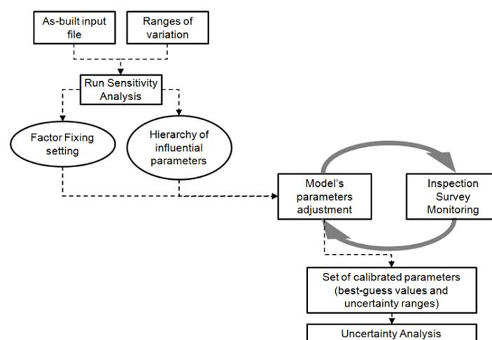
Figure 7-15: Main steps of the evidence-based calibration methodology
