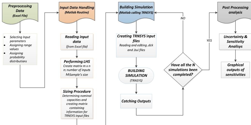
Figure 7-8: Monte Carlo simulation diagram flow
