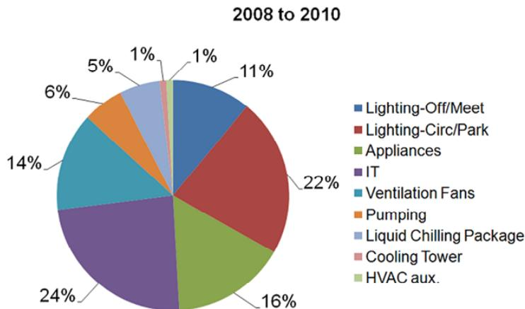
Figure 7-18: Whole-building electricity consumption disaggregation (at Level 4)
