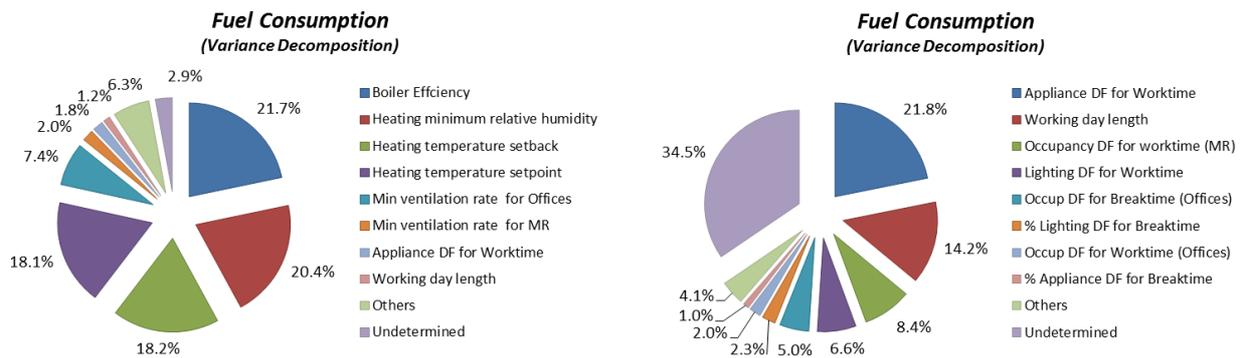
Figure 7-14: Whole building energy fuel consumption – Sensitivity indices for case 1 and 2 respectively
