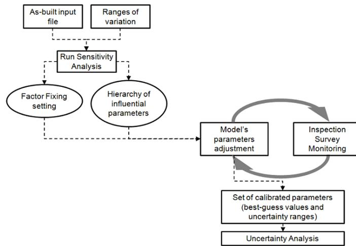
Figure 7-16: Main steps of the evidence-based calibration methodology
