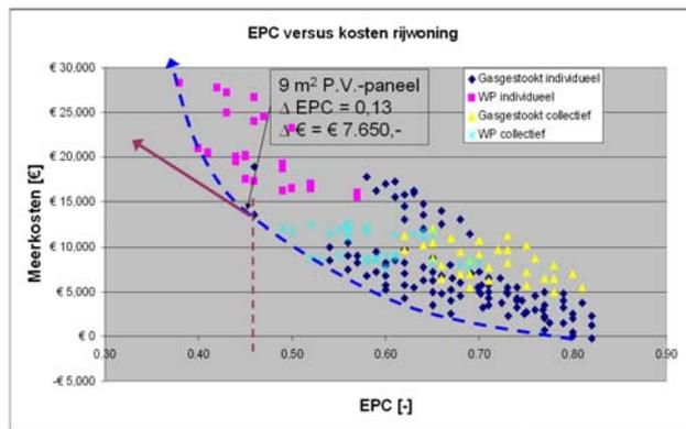
Figure 4.3 Additional cost versus EPC for integrated concepts
