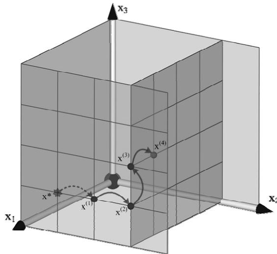
Figure 4.10. Illustration of the path of 4 orthogonal steps through a 3-dimensional parameter space to create 4 independent design parameter vector. The random base value,  $x^*$ , is used as a starting point for the process.
