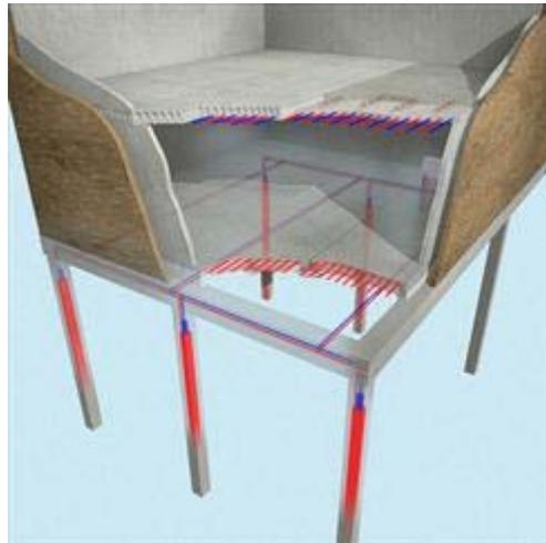
A consortium of Velta, Techneco and Betonson made it possible to combine the two proven concepts of Betonson's prefabricated thermo-active floor elements and energy piles into an energy-efficient heating and cooling system for dwellings. The system is complemented by a combination heat pump both providing space heating and hot water for domestic use.
