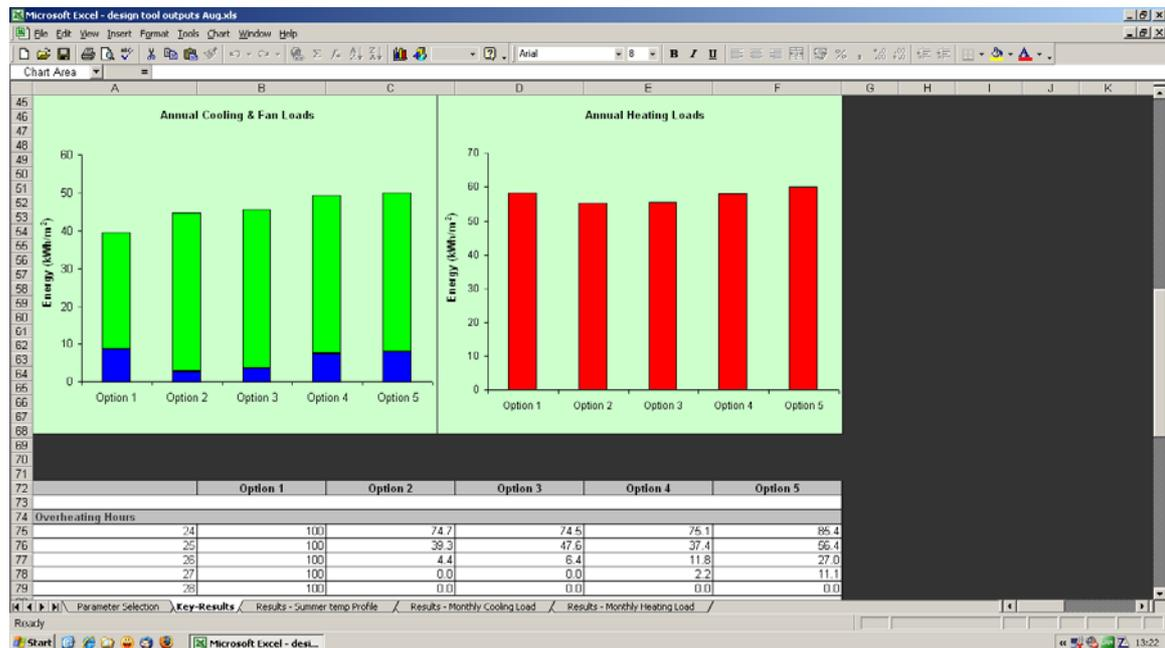
Figure 4.7 Key-results tab of the concept design tool TMAir where the energy consumption for cooling and heating are shown for the five selected options.
