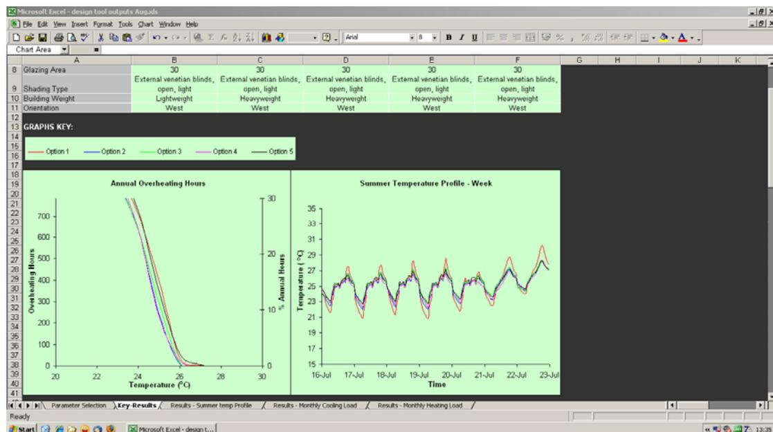
Figure 4.6 Key-results tab of the concept design tool TMAir where the annual overheating hours and the summer air temperature profile for a week are shown for the five selected options. The base-case building has input parameters exactly the same as the active thermal mass buildings.
