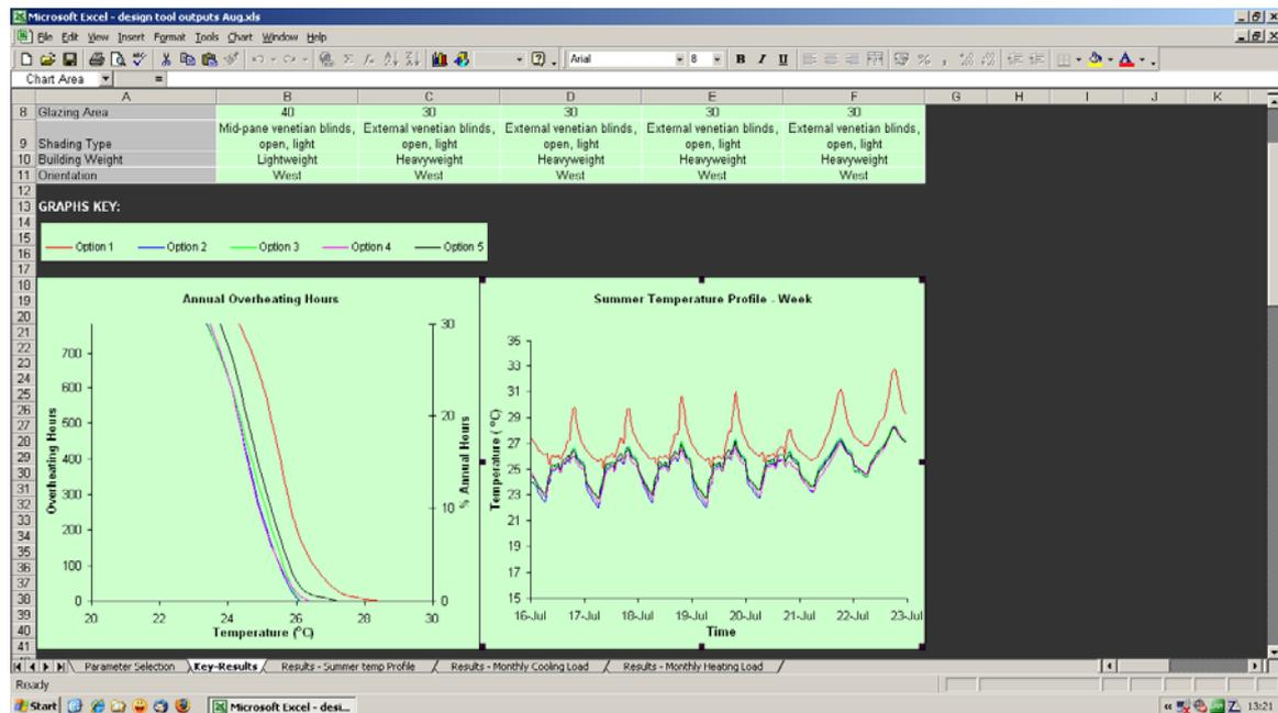
Figure 4.5: Key-results tab of the concept design tool TMAir where the annual overheating hours and the summer air temperature profile for a week are shown for the five selected options.
