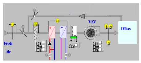
Figure 4: General view of a typical air distribution system.
