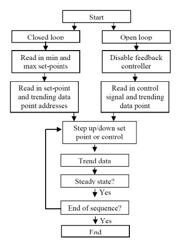
Figure 8b: Automated test signal generator.
