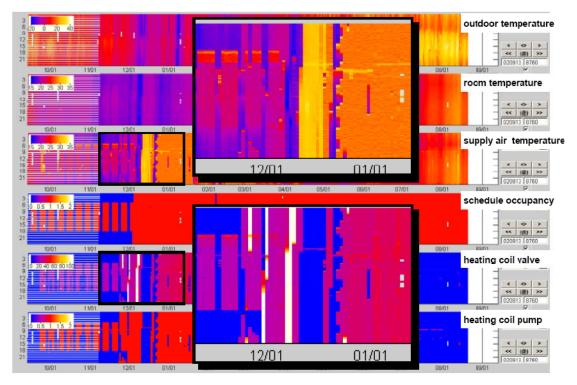
Figure 7a: Carpet plot of 6 data points for a time range of 11 months.
