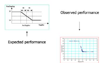
Figure 3: Verification of supply air temperature.
