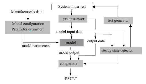
Figure 8a: Architecture of a model-based functional testing tool.
