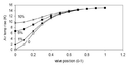
Figure 7: Heating coil air temperature rise as a function of valve position
