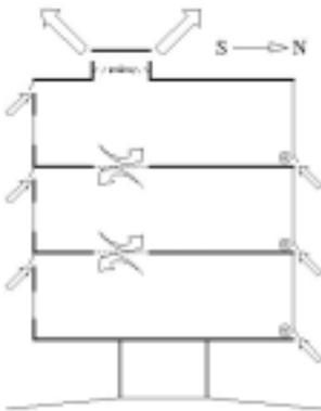
Figure 2: Principle of hybrid ventilation system (Aggerholm, 1999).
