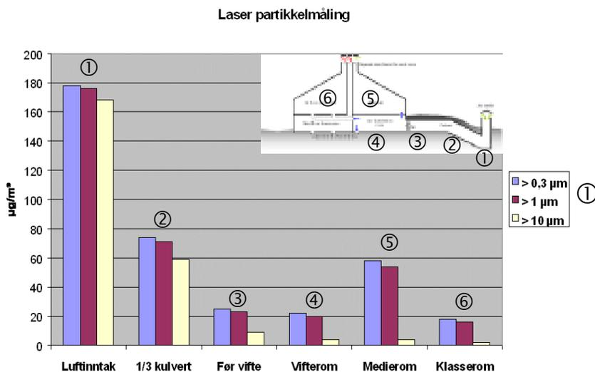
Figure 5: Gravimetric laser particle counter measurements of particles of different sizes at 6 different locations.
