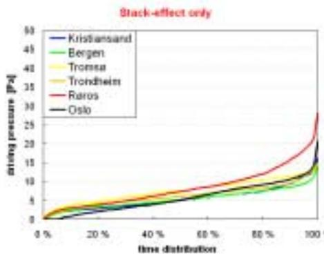
Figure 2a: Prevalent stack-effect driving forces.
