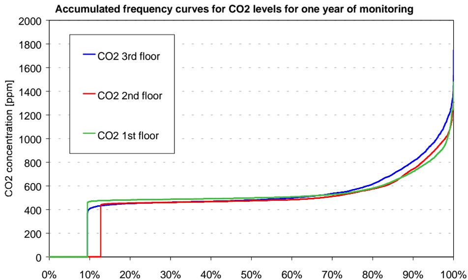
Figure 3: CO<sub>2</sub> levels at each office floor based on one year of monitoring. CO<sub>2</sub> concentrations are logged by the BEMS system. The figure shows average values for each floor from logging with two sensors at each floor.
