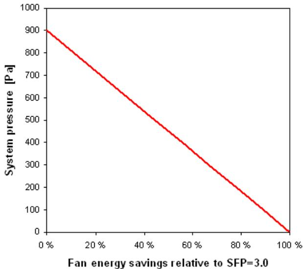
Figure 3: Fan energy savings for different system pressure losses, relative to a system with SFP=3.0.
