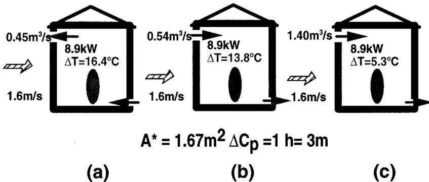
Figure 3: Three flow states in a building with identical ventilation parameters. The downward flow of  $0.54 \text{ m}^3/\text{s}$  is not stable, as shown by Li and Delsante (2000).
