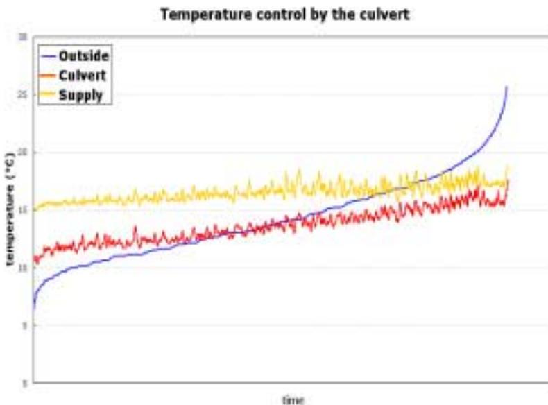
Figure 4b: Distribution curve showing the cooling effect culvert over a few months. “Culvert” is the air after it has passed through the culvert, “Supply” is the air after it has passed through the preheat battery.
