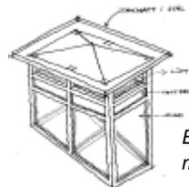
*Exhaust chimney, with motorised dampers at top*
