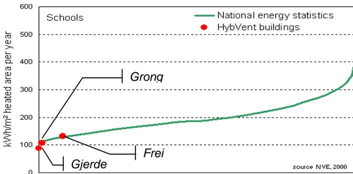
Figure 6: Distribution of specific energy consumption (not degree-day corrected) in kWh/m<sup>2</sup> heated area from the national database of energy consumption in 356 school buildings [7]. Three HybVent buildings are plotted as red dots.
