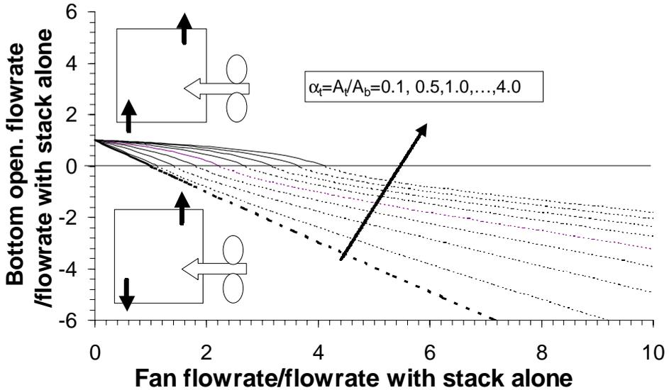
Figure 4: Flow rate through the bottom opening in a two-opening mixed-mode building with stack driven ventilation and a supply fan.
