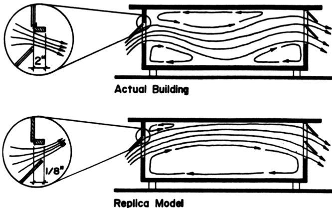
Figure 1: Different flow patterns obtained by wind tunnel tests when there were small changes in the inlet details. Note that the inner edge of the window was projected slightly inside the wall compared to the actual building (Smith, 1951).
