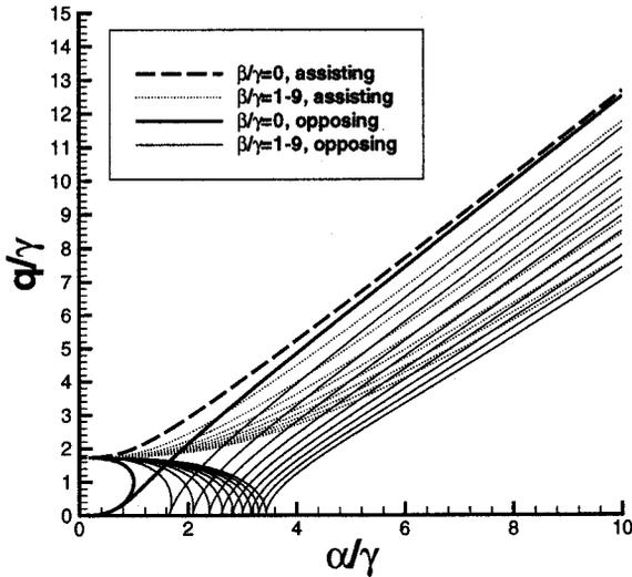
Figure 2: Ventilation flow rates for combined forces – both opposing and assisting winds. Where  $q$  is the ventilation flow rate,  $\alpha$ ,  $\beta$  and  $\gamma$  are the thermal buoyancy-, envelope heat loss- and wind- air change parameters, respectively. For a certain range of  $\alpha/\gamma$ , there are two stable solutions and one unstable solution.
