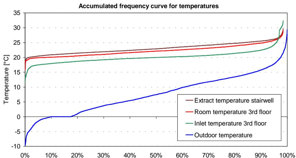
Figure 4: Average temperature levels at third floor. Temperature data are logged by the BEMS system from each temperature sensor. Average values are shown for the third floor.
