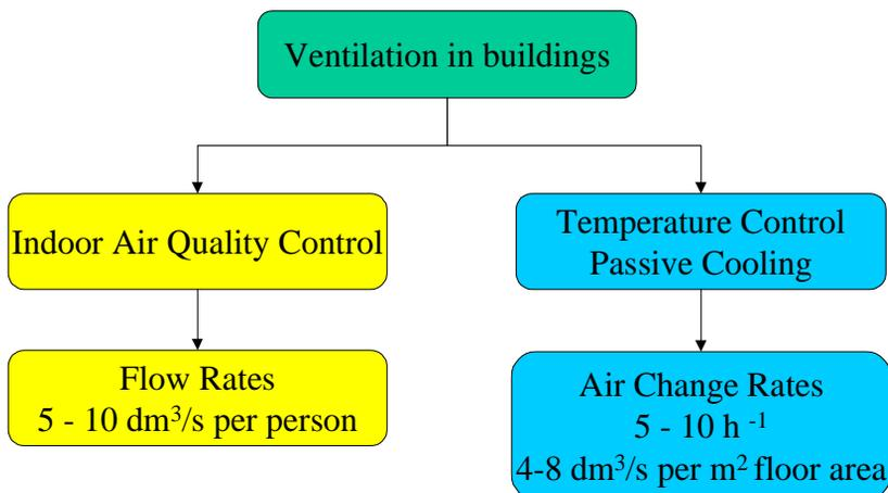
Figure 3: Functions of a ventilation system.
