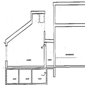
*cross-section showing principle of using double wall as supply shaft to classrooms*
