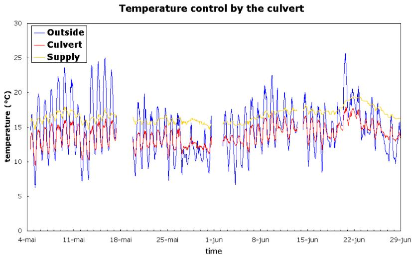
Figure 4a: The thermal performance of the culvert over a couple of months.
