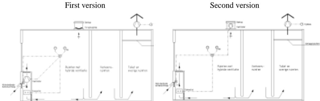
Figure 2. Scheme of ventilation system of Waterland school building.
