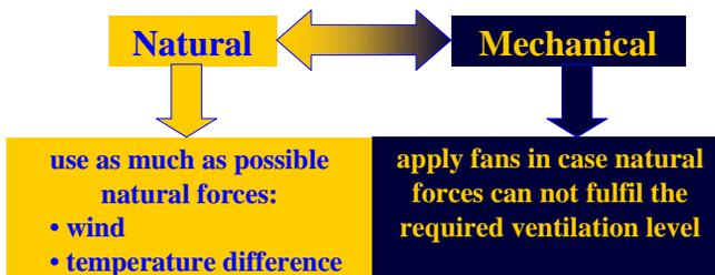
Figure 2: Schematic picture of hybrid ventilation.
