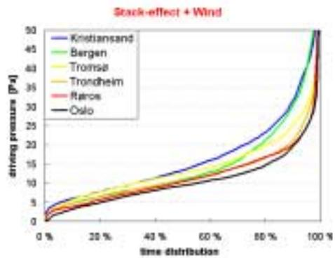
Figure 2b: Stack-effect driving forces.
