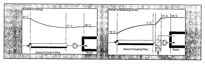
Figure 7 Principles of Ground Cooling and Heating
