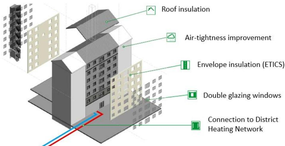
**Figure 44.** Diagram of the renovation measures undertaken. Source: VISESA, H2020 project “SmartEnCity” and Municipality of Vitoria-Gasteiz.
