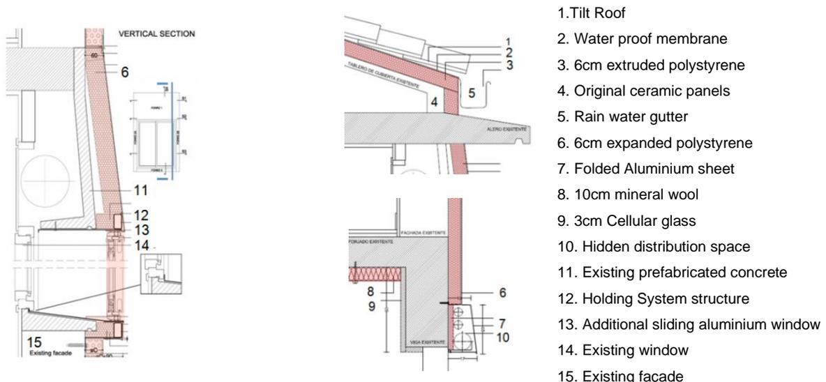
Figure 48. Construction details of renovation solution. Source: M.A.R. Arquitectos.
