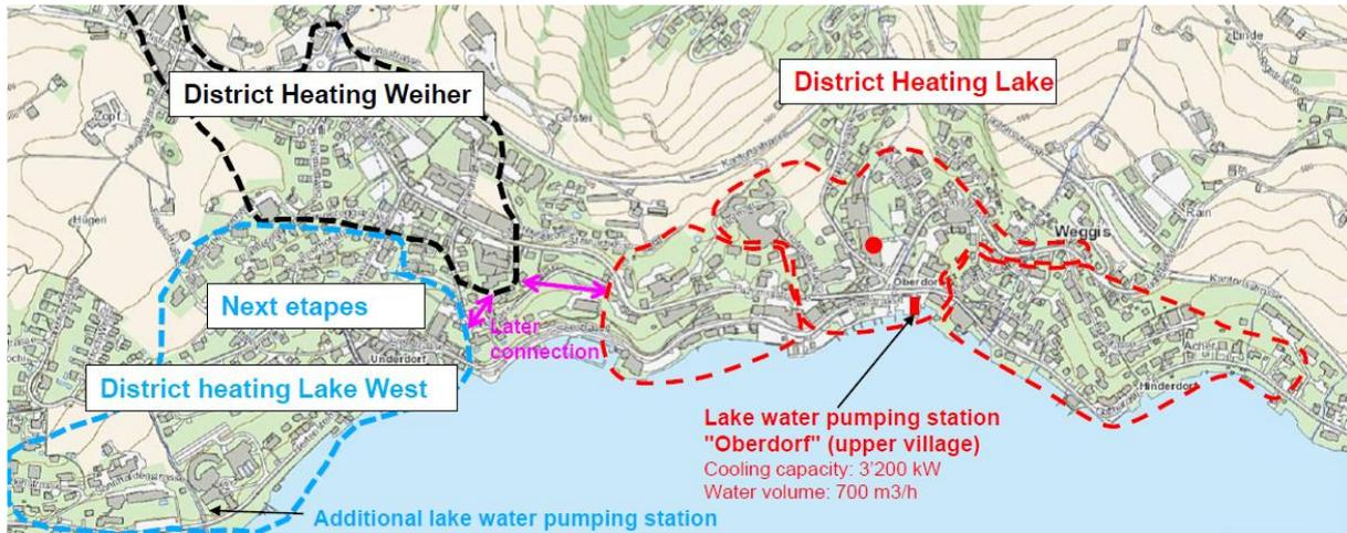
Figure 50. Schematic view of the different stages of the district heating networks in Weggis. Source: Corporation Weggis.
