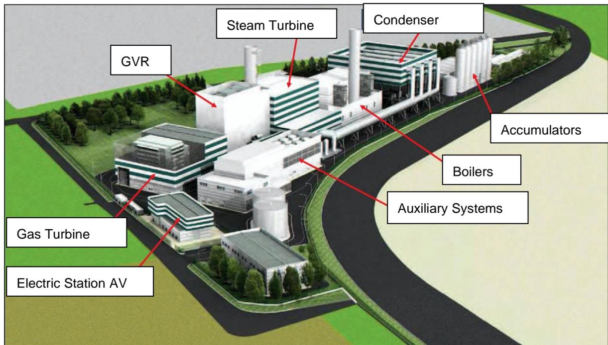
**Figure 25.** Schema of the new power station. Source: edited by the authors, based on Iren Energia S.p.A. report.
