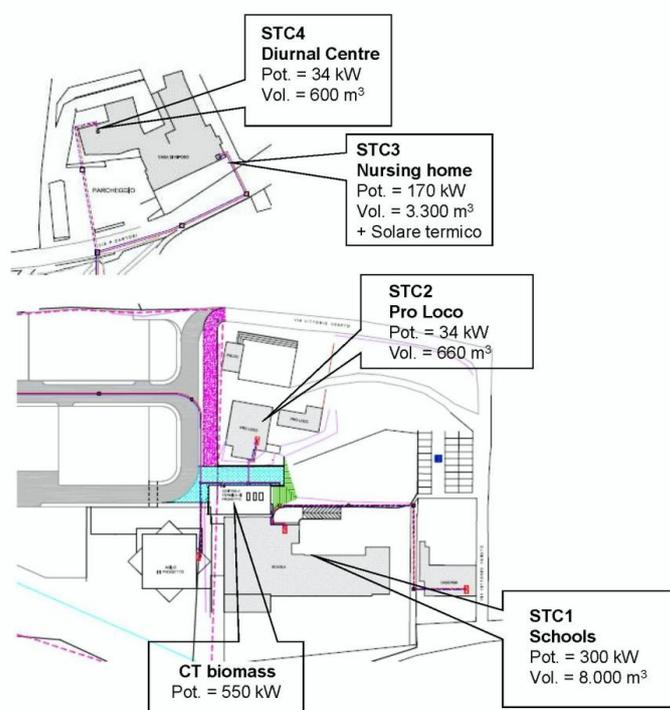
**Figure 21.** The district heating net includes 5 buildings: a CT thermal central station and 4 STC substations. For each building, a label describes the name of the station, the use, the installed power Pot, and the volume Vol. Source: technical drawing from as built project, by Comune di Valdastico.
