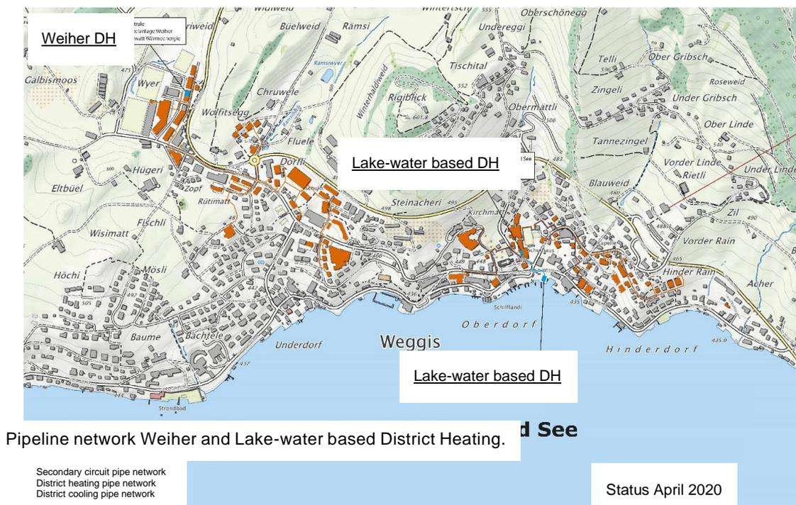
Figure 51. Schematic view of the building connected in April 2020 and existing pipeline network. Source: Corporation Weggis.
