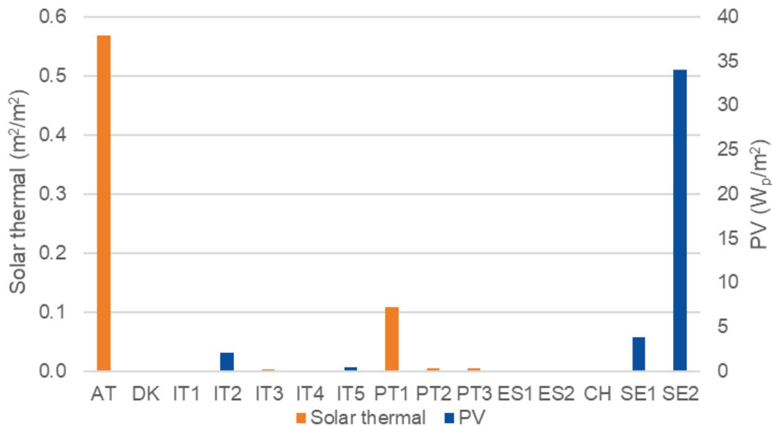
**Figure 63.** Size of the solar panels and PV installation, in relative terms, compared to the gross heated floor area.
