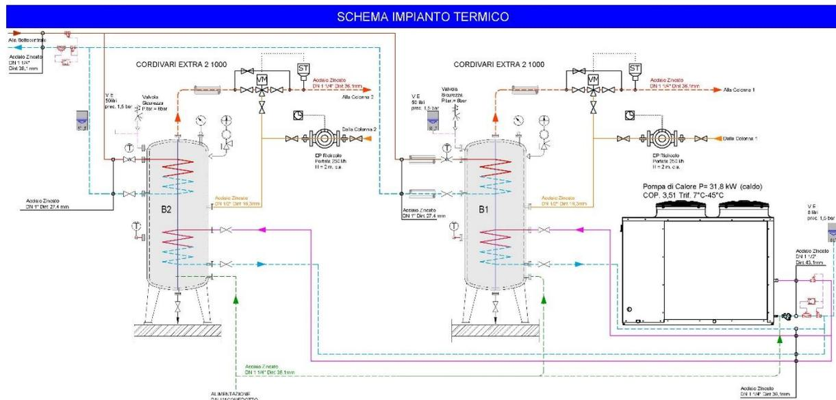
Figure 18. DHW system scheme. Source: ALER- Varese.
